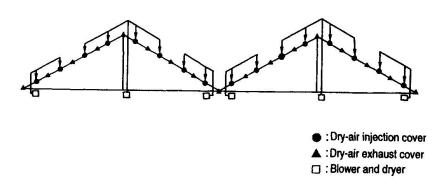
Fig. 3 Schematic drawing of dry-air injection system
