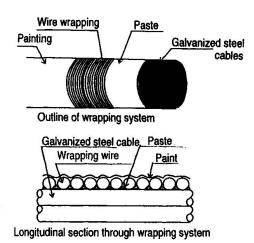
Fig. 1 Conventional cable protection system
