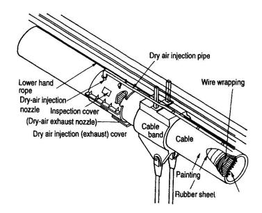
Fig. 2 Dry Air injection system (arrangement of pipes)
