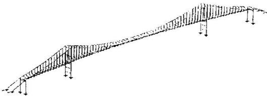
Fig. 6 Fish bone model of the bridge
