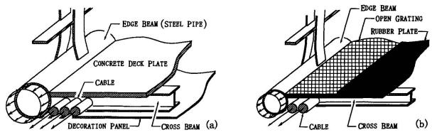
Fig.4 Cross-sections of the previously proposed steel structure (a), and the improved lighter steel one (b).
