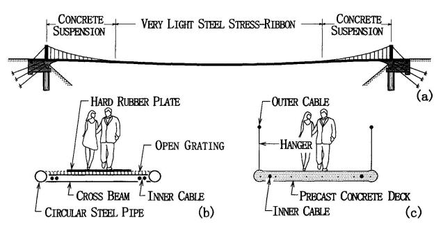
Fig.5 The proposed hybrid stress-ribbon pedestrian bridge. The elevation (a); the cross-section of the central portion of steel stress-ribbon deck (b); that of concrete suspension deck close to the abutment (c).
