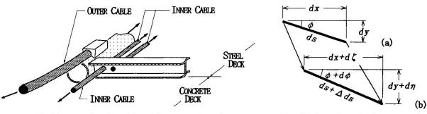
Fig.6 Inner and outer cables at the connection of steel and concrete decks.
