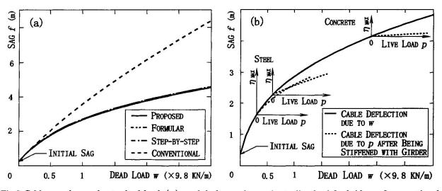
Fig.8 Cable sag change due to dead load (a), and deck sag change due to live load for bridges of conventional concrete, previously proposed steel and proposed lighter steel constructions (b).
