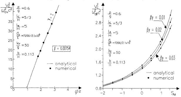
Fig.2: Critical wind speed versus frequency ratio p.
