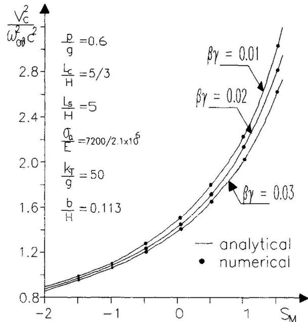
Fig.2: Critical wind speed versus frequency ratio  $\phi$ .
