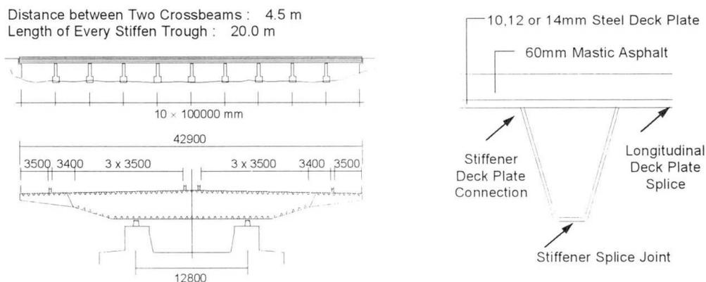
Fig. 1 Example bridge and its orthotropic deck
