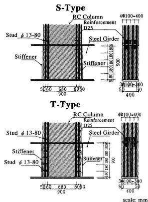
Fig. 1. Detail Specimens
