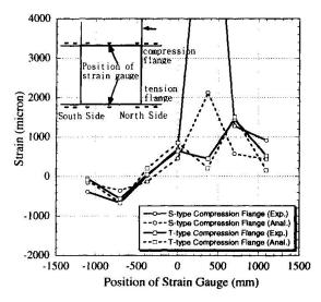
Fig. 4. Strain Distribution on Compression Flange for Each Type
