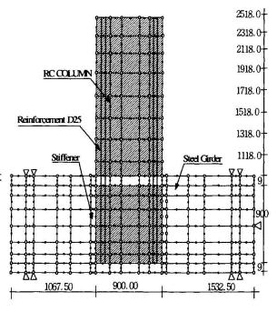
Fig. 2. Mesh generation of FEM
