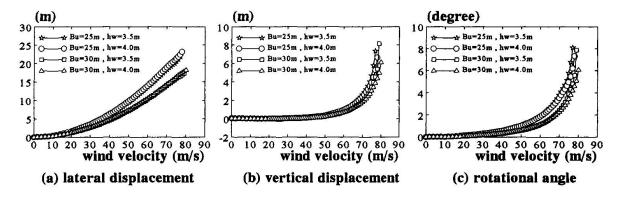
Figure 3: Displacement at the middle of the center span (after completion)
