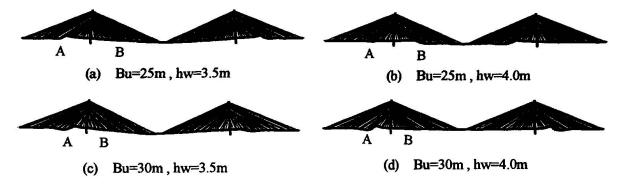
Figure 2: Incremental displacement at ultimate state
