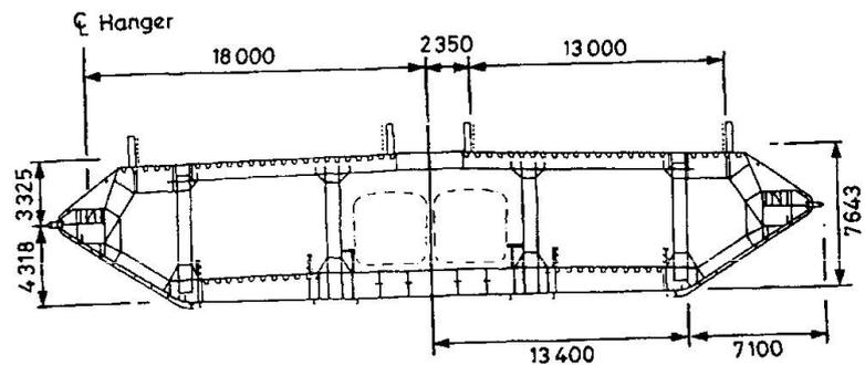
Figure 1 Typical Cross-section of Deck Unit (Beard 1993)
