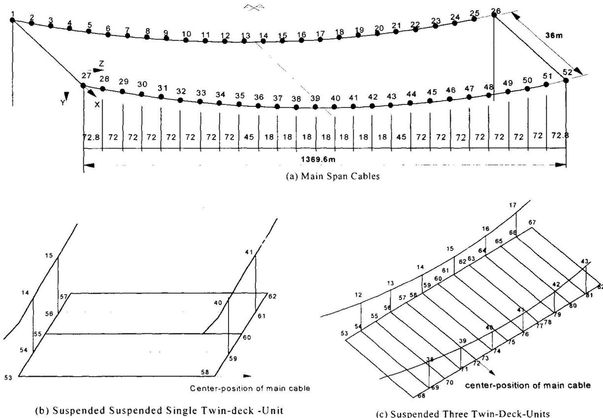
Figure 3 Finite Element Models with Node Numbering
