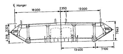
Figure 1 Typical Cross-section of Deck Unit (Beard 1993)
