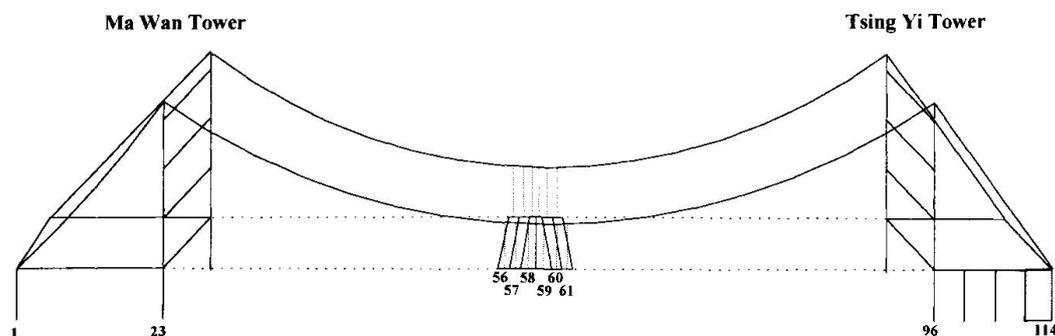
Figure 2 Number System of Deck Units
