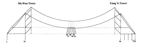
Figure 2 Number System of Deck Units
