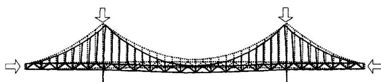
Fig. 1 Dead load deformation due to large axial force
