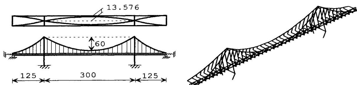
*Fig. 2 A Self-Anchored Suspension Bridge*
