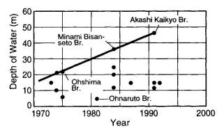
Fig. 7 Development of Underwater Foundation in Japan
