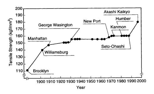
Fig. 14 Increase in Strength of Cable Wire
