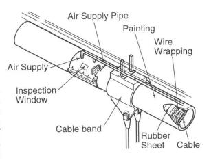
Fig. 17 Corrosion Protection System of Main Cable
