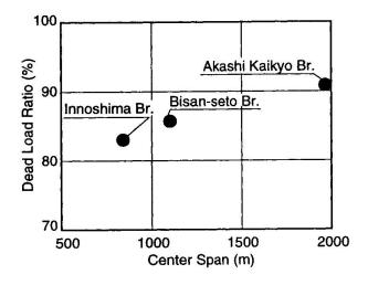
Fig. 12 Dead Load Ratio in Cable Tension Force
