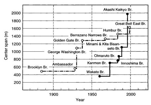
Fig. 2 History of Span Enlargement of Suspension Bridge
