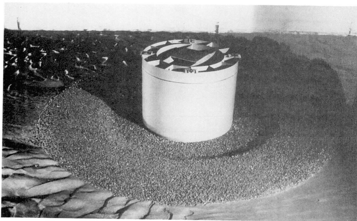
Photo 1 Scouring Test with Protection
