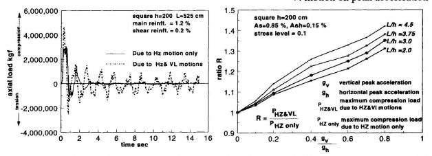
Fig. 7 Effect of vertical motion on axial load response of RC pier
