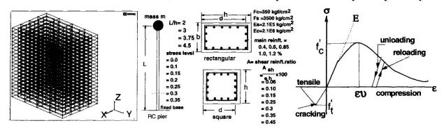
Fig. 1 A) 3D model b) Parameters of the study Fig. 2 Modeling of concrete in compression
