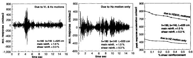
Fig. 5 (a, b) Effect of V. motion on HZ acceleration response V. motion on peak acceleration
