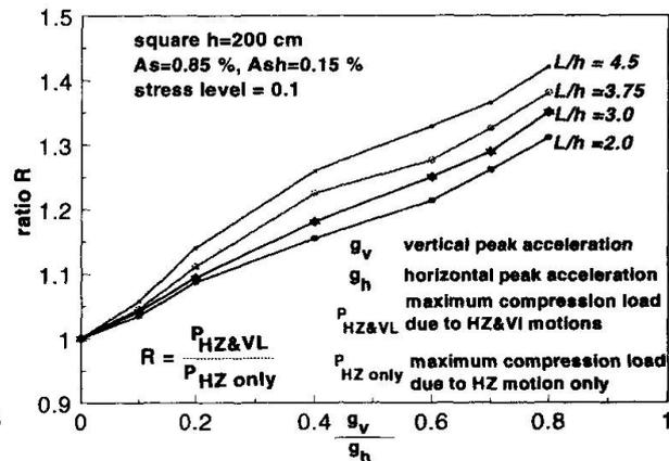
Fig. 7 Effect of vertical motion on axial load response of RC pier
