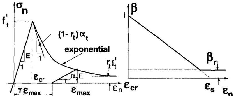
Fig. 4 a) Tension stiffening b) Retention factor
