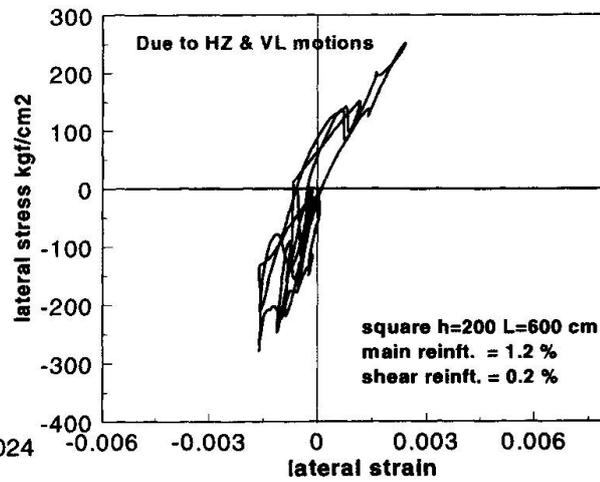
Fig. 13 (a, b) Effect of vertical motion on lateral stress strain for RC pier
