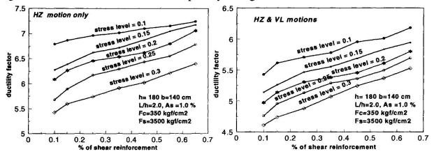
Fig. 9 (a, b) Ductility of piers with different ratios of shear reinforcement and stress level
