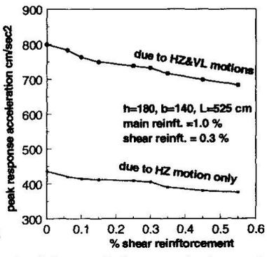
Fig. 5 (a, b) Effect of V. motion on HZ acceleration response
