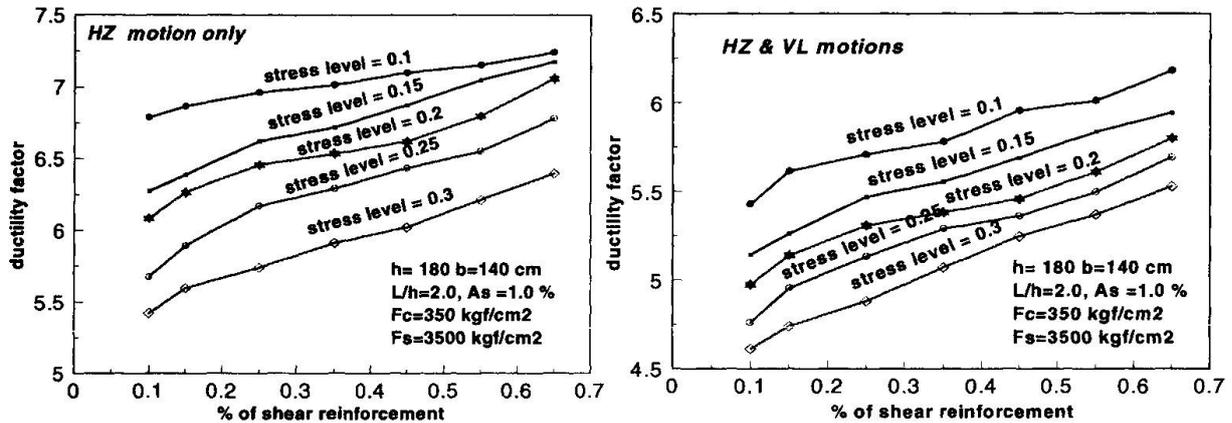
Fig. 9 (a, b) Ductility of piers with different ratios of shear reinforcement and stress level
