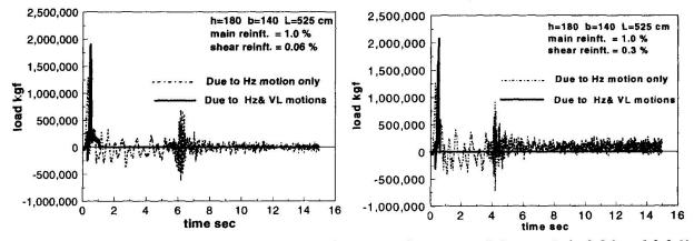
Fig. 10 (a, b) Effect of vertical motion on load capacity for ratios of shear reinft. 0.06 and 0.3 %
