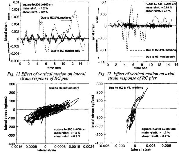
Fig. 13 (a, b) Effect of vertical motion on lateral stress strain for RC pier Case A HZ motion only Case B HZ & VL motions.
