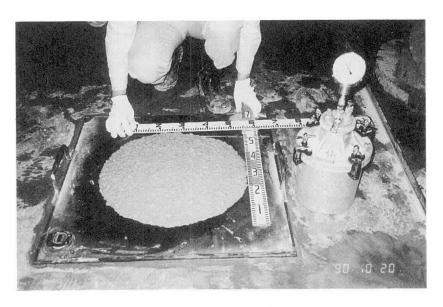
Photo 2 Slump Test of Antiwashout Underwater Concrete
