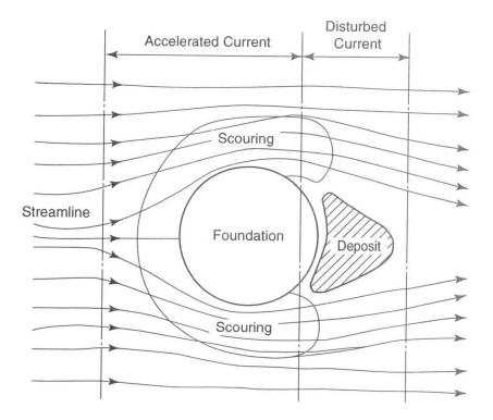
Fig. 9 Concept of Flow around Foundation
