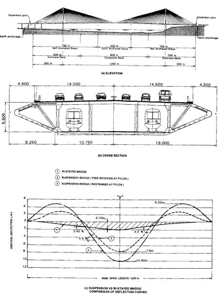
Fig. 6 Exemple of 1,200 m. Bi-stayed Bridge
