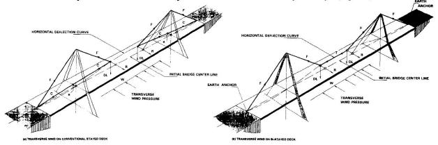
Fig. 7 Wind on decks: Pendulum Analogy
