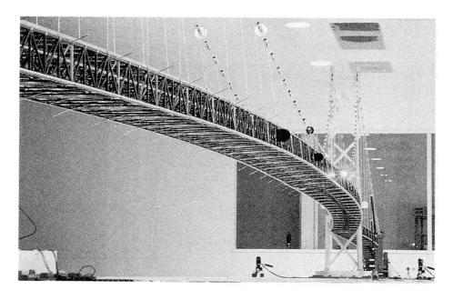
Photo 3 Displacement of the Akashi Kaikyo Bridge in Wind Tunnel Test
