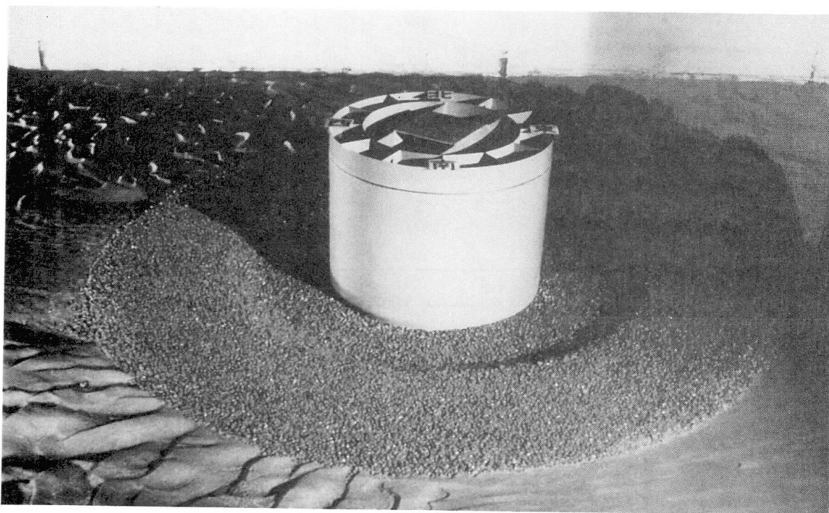
Photo 1 Scouring Test with Protection
