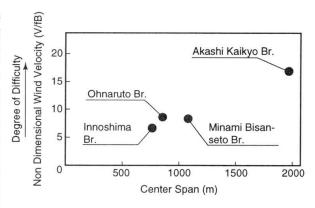
Fig. 11 Degree of Difficulty to Keep Aerodynamic Stability
