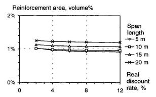
Fig. 7 Optimal reinforcement area in % of concrete volume.
