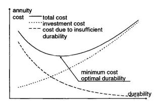
Fig. 1 Optimal durability occurs at minimum total cost, the sum of investment cost and cost due to insufficient durability.
