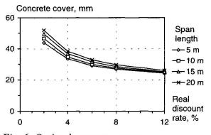
Fig. 6 Optimal concrete cover.
