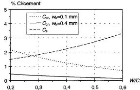
Fig. 2 Measured chloride threshold values and maximum surface chloride concentrations by water binder ratio. Redrawn from /8/.
