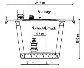
Fig. 4: Cross section, approach bridge
