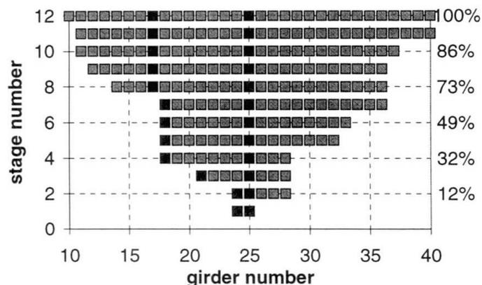
Figure 1 Deck configurations studied. Light grey: hinged segments; dark grey: accelerometers location. The percentage of completion is indicated on the right ordinate.
