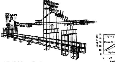
Fig.10 Scheme of load test apparatus (scale 1: 24)
