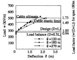
Fig.9 Load vs deflection by finite deflection analysis
