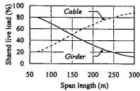
Fig.7 Load shared by girder and cable
