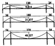
Fig.2 Structure profile shapes derived by stated rationale for varying span lengths
