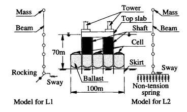
Fig.3 Lumped mass model for dynamic analysis
