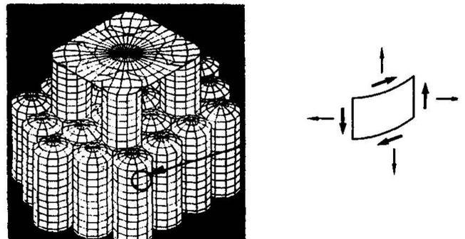
Fig.4 Structural behavior under seismic effects
