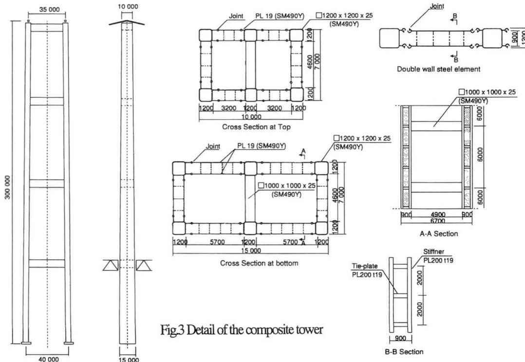
Fig.3 Detail of the composite tower
