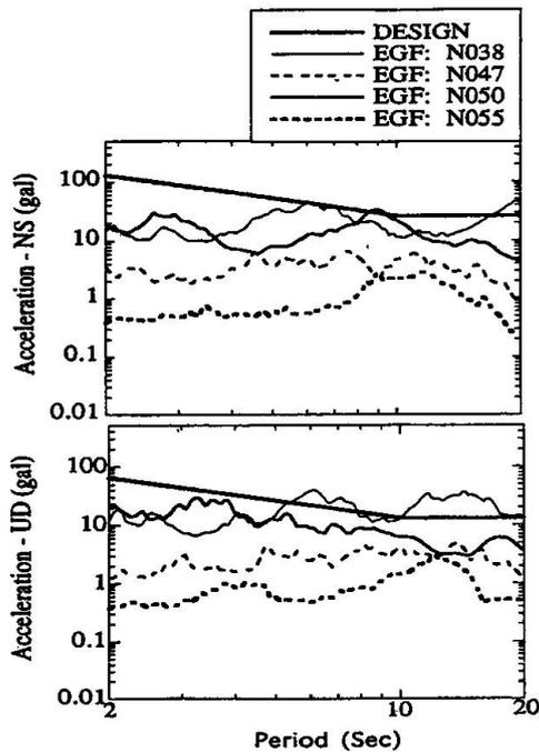
Fig. 7 Acceleration response spectra of synthetic signals induced by B model on the Nankaido Trough ( $h=2\%$ ) compared with the design spectra for the Akashi Kaikyo Bridge. Components NS (top), and UD (bottom)
