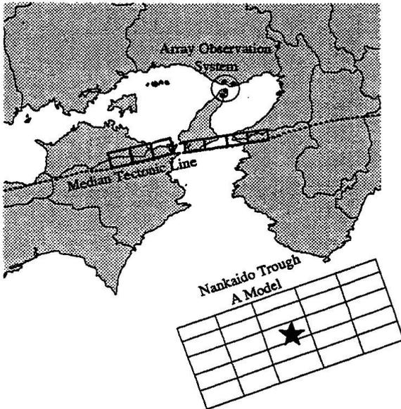
Fig. 3 Assumed two-fault-plane source mechanism on the MTL, along with the A model source mechanism on the Nankaido Trough.
