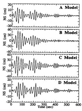
Fig. 6 Synthetic displacement time histories at Akashi Station induced by the Nankaido Trough. Event N038 is used as Green's function for each source model.
