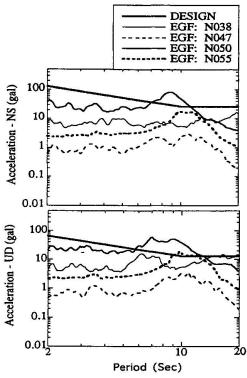
Fig. 5 Comparison of the acceleration response spectra of synthetic signals induced by the MTL (h=2%) with the design spectra for the Akashi Kaikyo Bridge.
