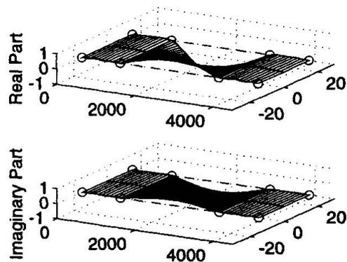
Fig. 5 Root locus of uncontrolled bridge and flutter mode shapes.
