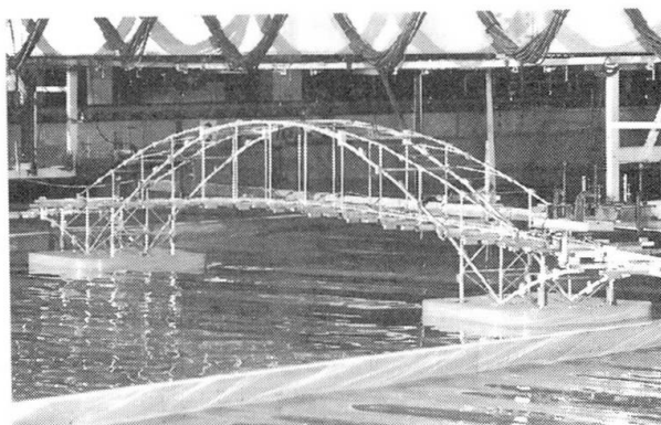
Photo. 3 In-wave elastic model experiment (Scale: 1/40)
