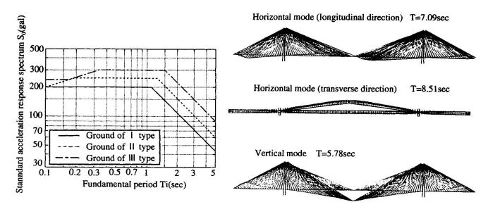
Fig.9 Acceleration response spectrum
