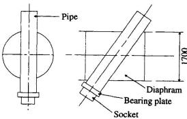
Fig.12 Anchor part for cables
