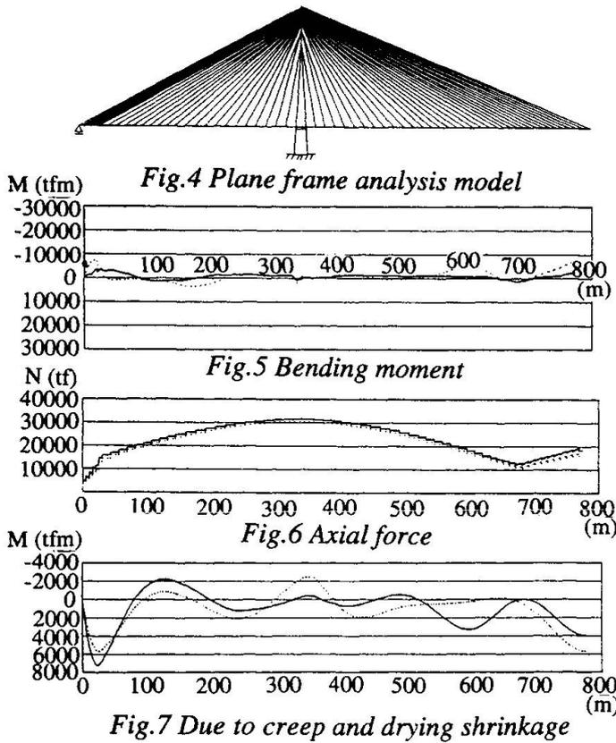
(2) Effect of creep and drying shrinkage
