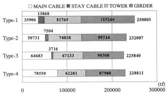
Fig. 3 Comparison of weight of steel
