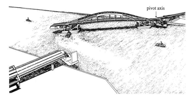
Fig. 5 Swinging Procedure
