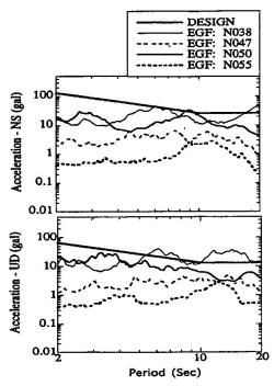
Fig. 7 Acceleration response spectra of synthetic signals induced by B model on the Nankaido Trough (h=2%) compared with the design spectra for the Akashi Kaikyo Bridge.
