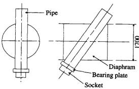
Fig.12 Anchor part for cables
