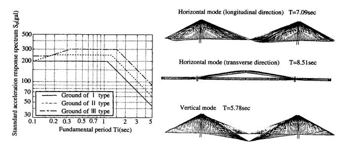
Fig.9 Acceleration response spectrum
