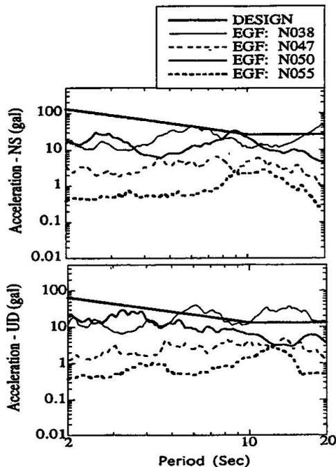
Fig. 7 Acceleration response spectra of synthetic signals induced by B model on the Nankaido Trough ( $\eta=2\%$ ) compared with the design spectra for the Akashi Kaikyo Bridge. Components NS (top), and UD (bottom)
