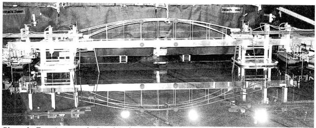
Photo. 1 Experiment on the Riged-Body Model Motions in a Large-Scaled Water-tank
