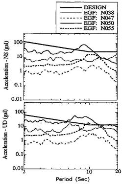
Fig. 5 Comparison of the acceleration response spectra of synthetic signals induced by the MTL (h=2%) with the design spectra for the Akashi Kaikyo Bridge.
