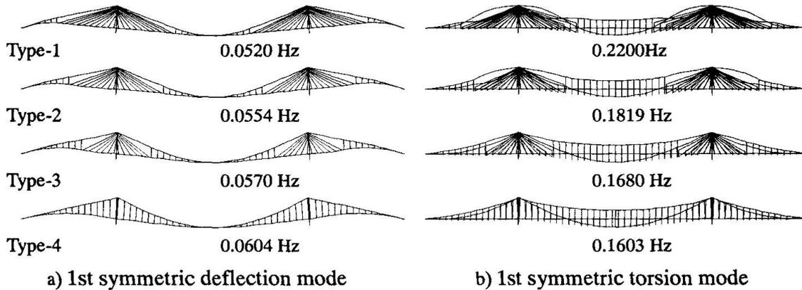
Fig. 4 Basic modes by natural vibration analysis
