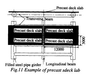
(1) Deck slab and frame structure Figure 11 shows an example of precast PC deck slab. As the deck slab used for 2 main girder section, RC deck slab, PC deck slab and composite steel slab may also be adopted. However, precast PC deck slab is the most appropriate choice because the construction term could be shortened and the effects of creep and drying shrinkage are small.
