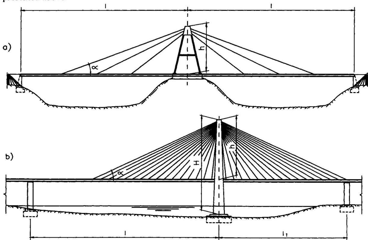
Fig. 2 Cable-stayed bridge having one pylon and two spans.
