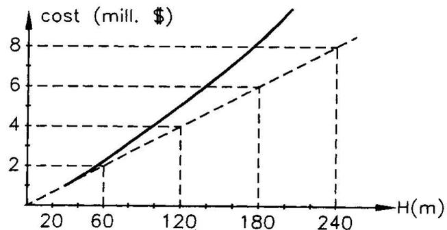
Fig. 3 Pylon cost-height diagram
