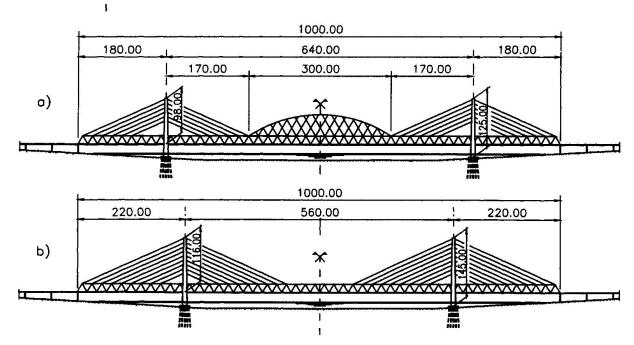
Fig. 6 Comparative cable-stayed bridge solutions
