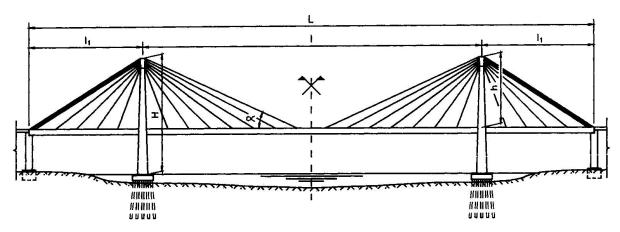
Fig. 1 Cable-stayed bridge having two pylons and three spans
