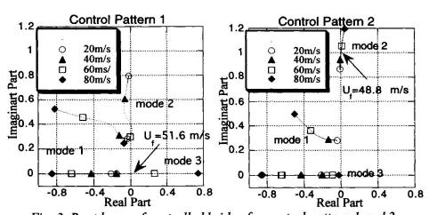
Fig. 3 Root locus of controlled bridge for control pattern 1 and 2.
