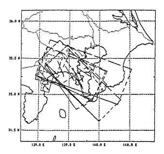
Fig.1 Fault Plane Models Proposed for 1923 Kanto Earthquake
