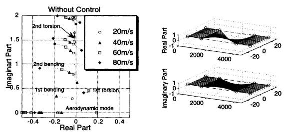
Fig. 5 Root locus of uncontrolled bridge and flutter mode shapes.
