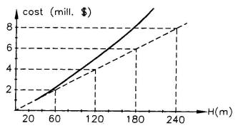
Fig. 3 Pylon cost-height diagram
