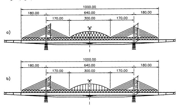
Fig. 4 Cable-stayde bridge stiffened by means of a middle arch. Elevation
