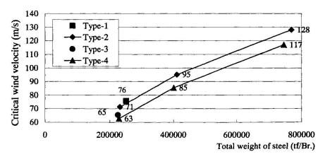
Fig. 5 Relationship between critical wind velocity and weight of steel
