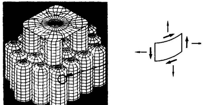
Fig.4 Structural behavior under seismic effects
