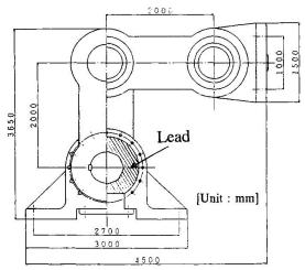
(a) Rotational Lead Extrusion Damper
