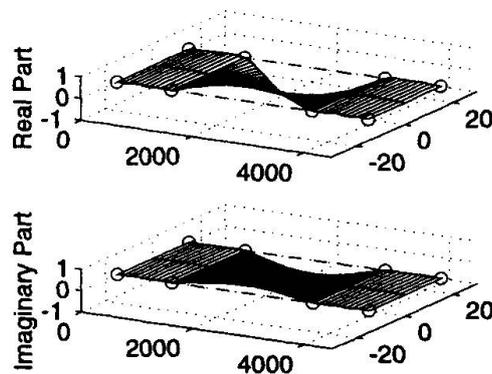
Fig. 5 Root locus of uncontrolled bridge and flutter mode shapes.
