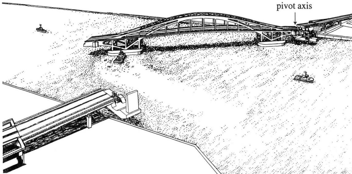
Fig. 5 Swinging Procedure
