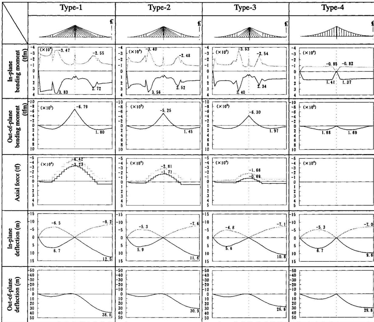
Fig. 2 Member-end forces and deformations of main girders
