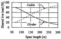
Fig.7 Load shared by girder and cable
