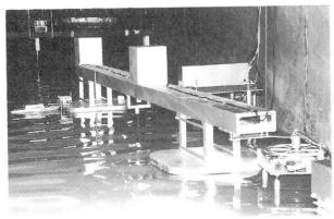
Photo. 2 Swinging and temporary mooring experiment (Scale: 1/80)
