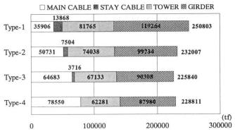
Fig. 3 Comparison of weight of steel
