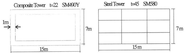
Fig.2 Cross sections of composite and steel towers
