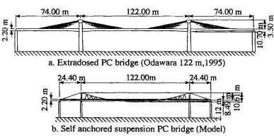
Fig.1 Prestressed concrete (PC) bridges with tendons of large eccentricity
