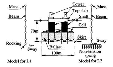
Fig.3 Lumped mass model for dynamic analysis
