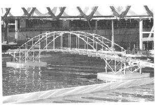
Photo. 3 In-wave elastic model experiment (Scale: 1/40)
