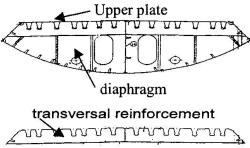
Fig. 1 Section of the railway deck and transversal reinforcement
