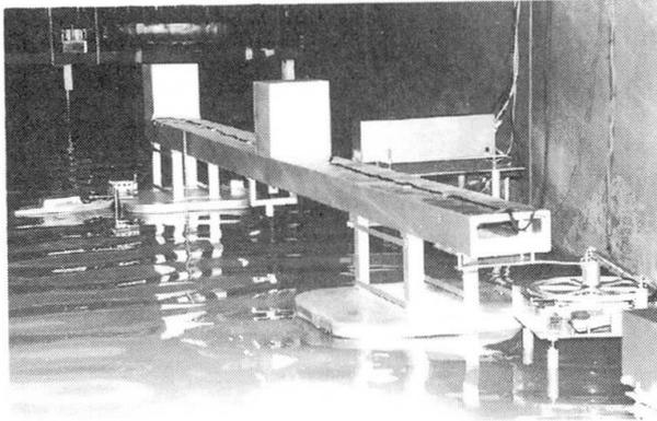
Photo. 2 Swinging and temporary mooring experiment (Scale: 1/80)
