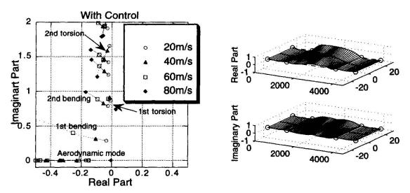
Fig. 6 Root locus of controlled bridge and flutter mode shapes.
