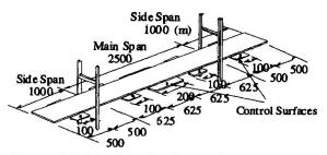
Fig. 4 Model of the bridge with position of control surfaces.
