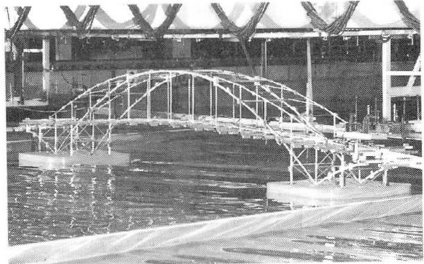
Photo. 3 In-wave elastic model experiment (Scale: 1/40)
