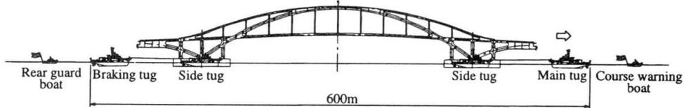
(STEP 3) The floating bridge is connected to the mooring equipment via tug winch operation.
