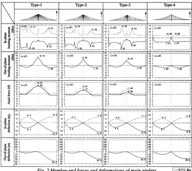
Fig. 2 Member-end forces and deformations of main girders
