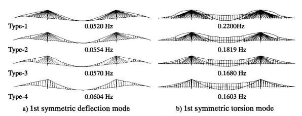
Fig. 4 Basic modes by natural vibration analysis
