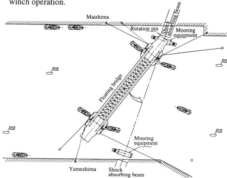
Fig. 6 Erection Steps
