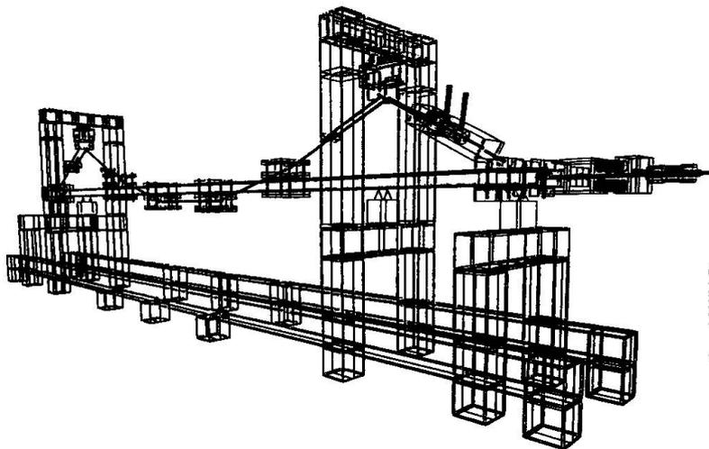
Fig.10 Scheme of load test apparatus (scale 1: 24)
