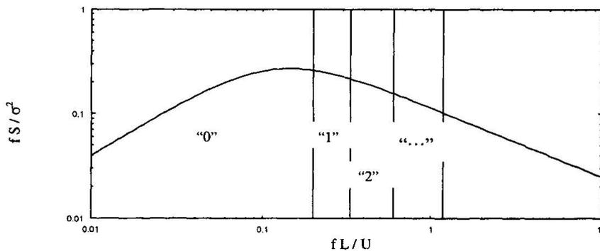
Figure 13 Normalised wind spectrum divided in frequency sub-ranges
