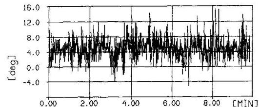
Figure 11 Incidence angle of wind speed measured on Humber bridge, from (Bocciolone et al.)
