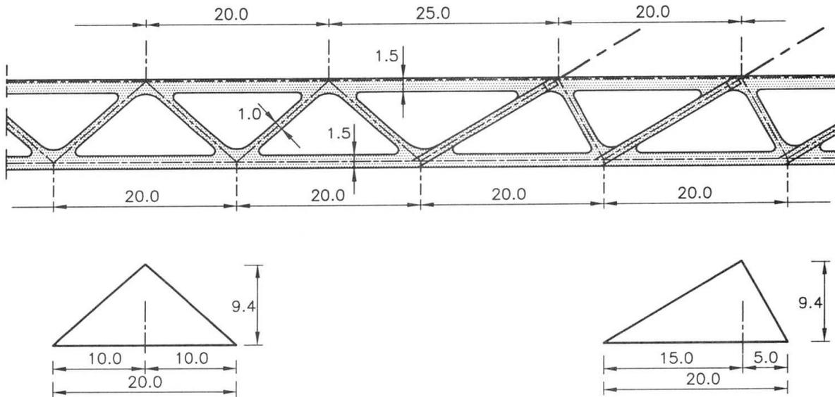
*Fig.11 Change of truss geometry*
