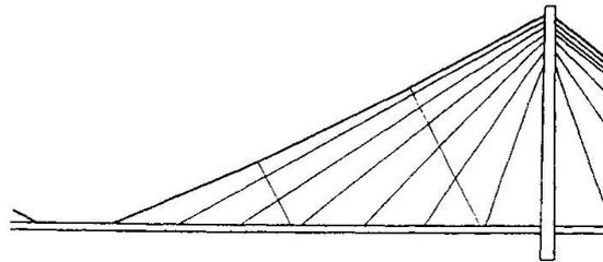
*Fig.9 Secondary stabilizing cables stressed against the top stay cable*
