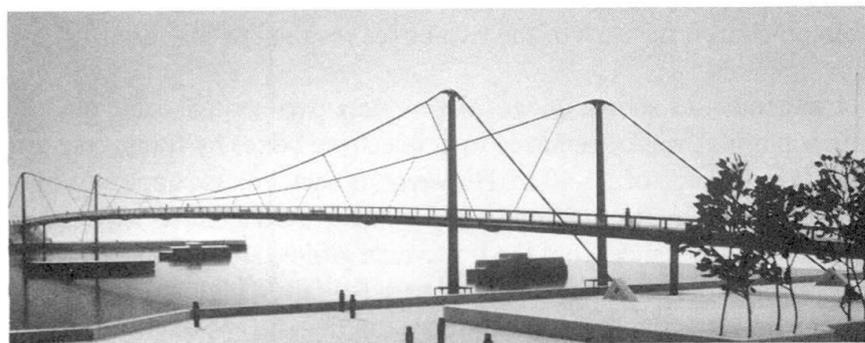
*Fig.6 Design for a pedestrian bridge across the Thames in London. Free-standing column pylons with axial compression due to orientation of the backstays in the vertical plane defined by the pylon axis and the adjacent main span cable tangent (Millennium Bridge Competition 1996)*
