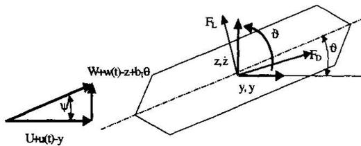
Figure 10 Variables defining wind forces on the deck
