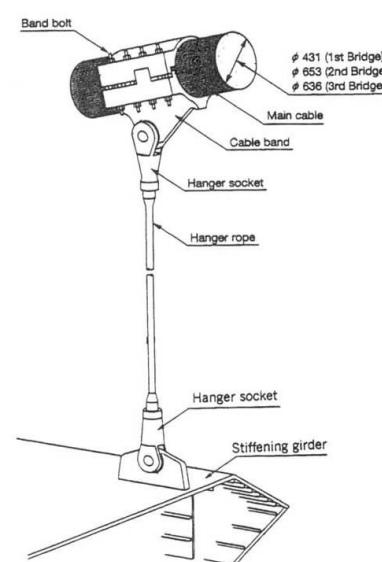
*Fig.3 Hanger rope fixing structure*
