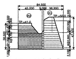
Fig.2 Planned Lifts for Construction
