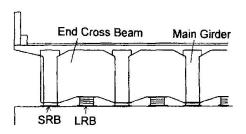
Fig. 3 LRB-SRB Isolation System
