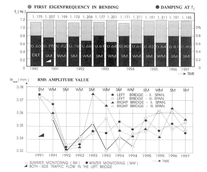
Fig.9 Changes in relative frequency, damping and displacement RMS amplitude values, 1990 - 1997
