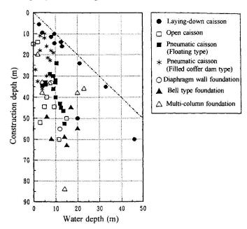
Fig. 1 Completed deep water foundation executions
