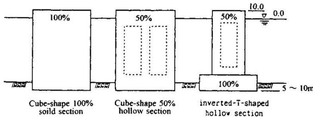
Fig. 4 Laying-down caisson used for the trial calculation
