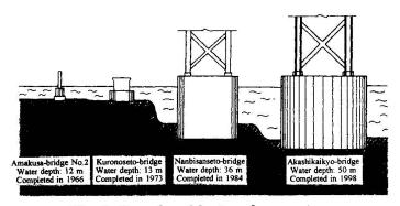
Fig. 2 Completed laying-down caissons
