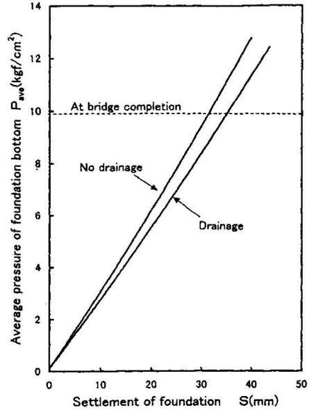
Fig. 8 Main tower foundation settlement forecast analysis
