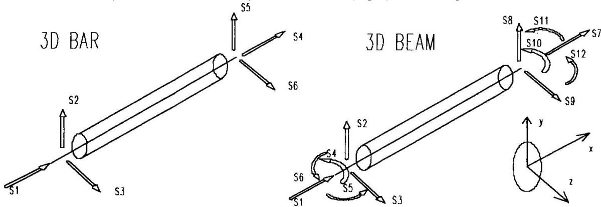
Fig.1: The 3D bar and beam member
