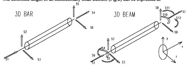
Fig. 1: The 3D bar and beam member
