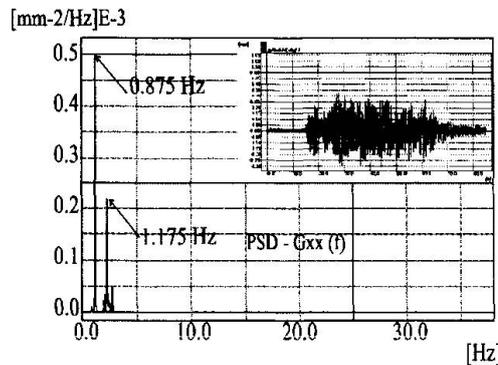
Fig. 6 PSD at point 039 caused by TATRA 815
