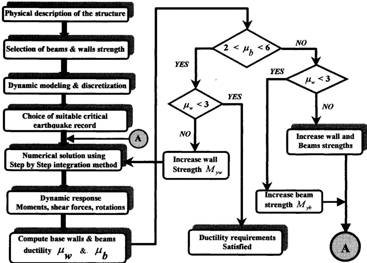
Fig. 4. Flowchart for dynamic inelastic analysis procedure
