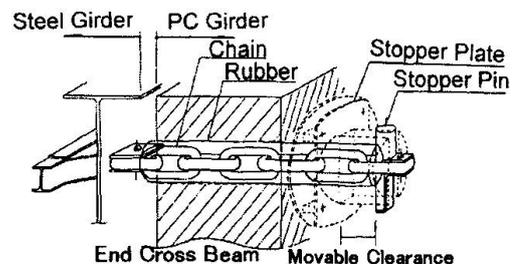
*Fig. 5 Restrainer with Rubber-sheathed Chain*
