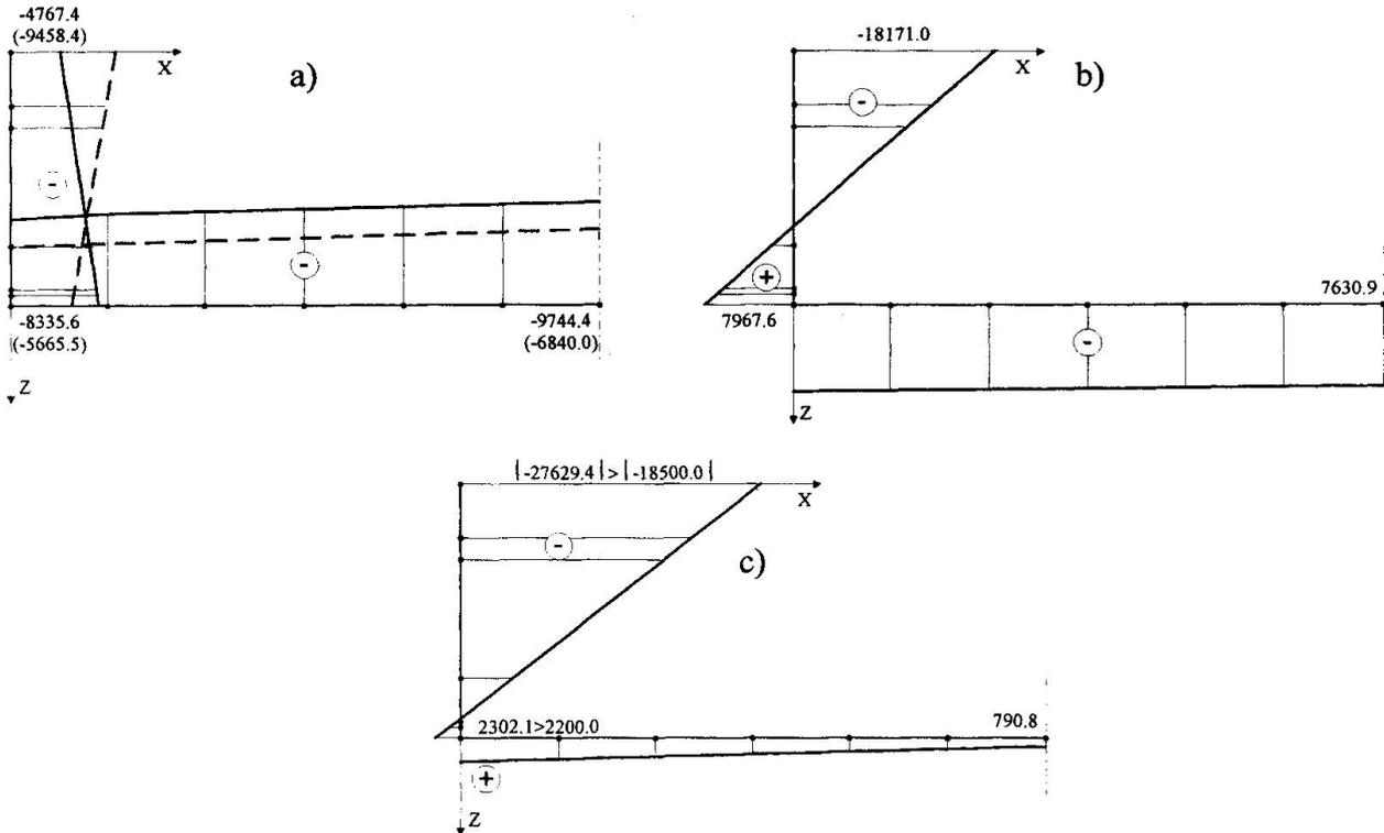
Fig. 4 Diagrams of stress  $\sigma_y$  in the middle of girder span length, (a) effect of own weight and prestressing in  $t_0$  and  $t_\infty$  (b) effect of live loading, (c) effect of own weight, prestressing and live loading in  $t_\infty$
