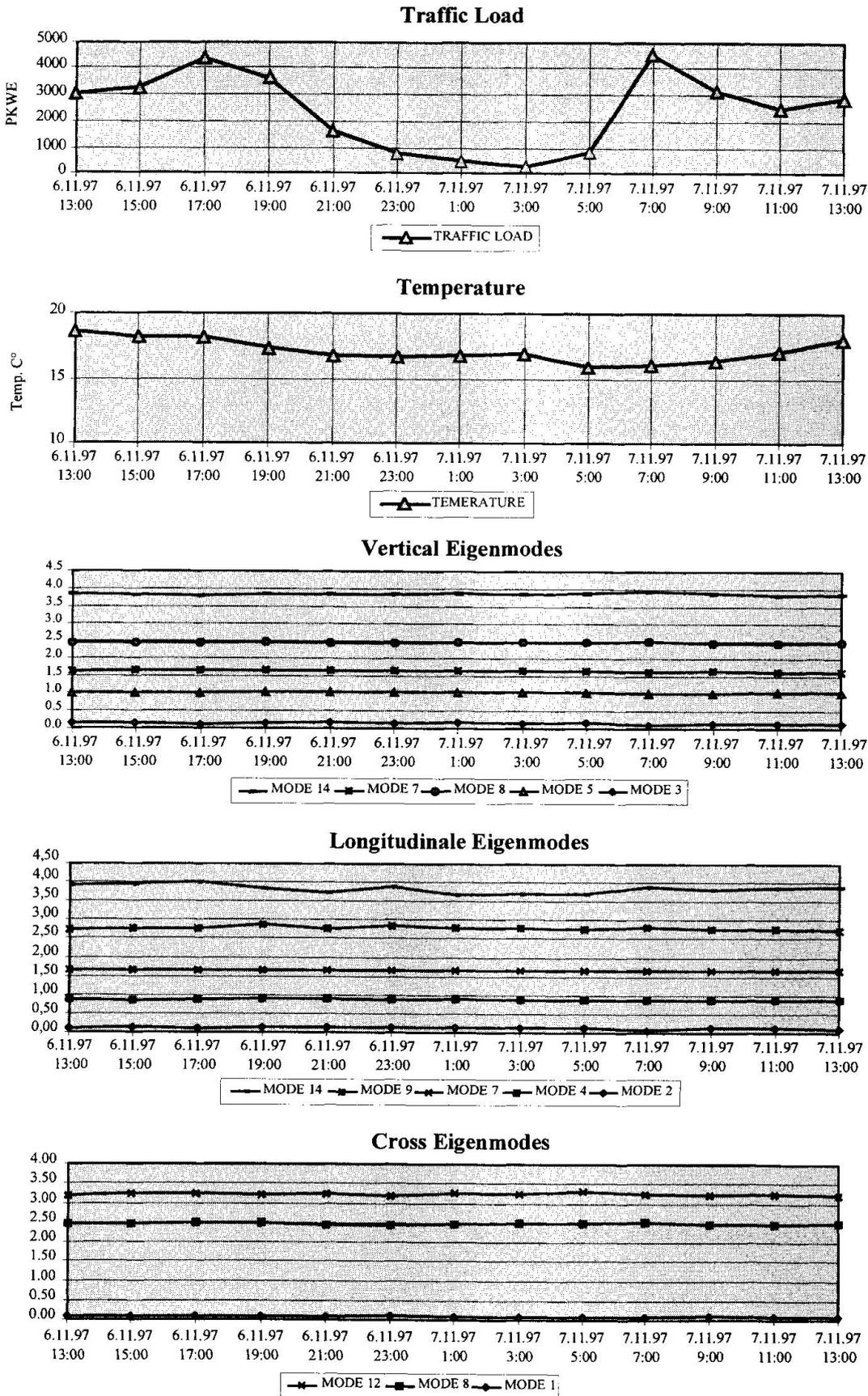
Fig. 3 24 hour test results, traffic load, temperature, frequencies
