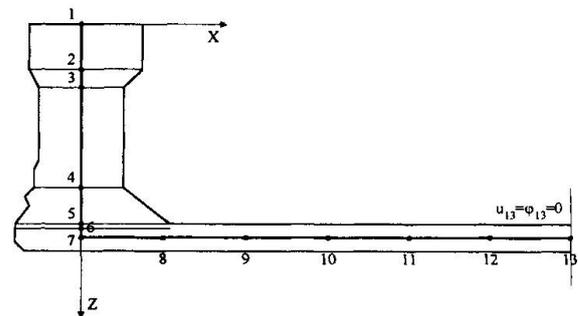
Fig. 3 Mesh of finite strips and symmetry conditions
