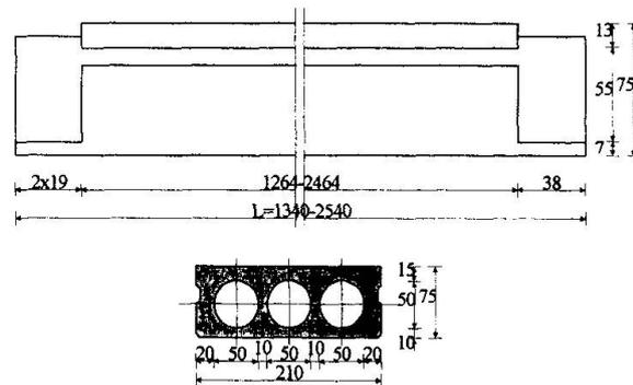
Fig. 5 View and cross-section of bridge girder
