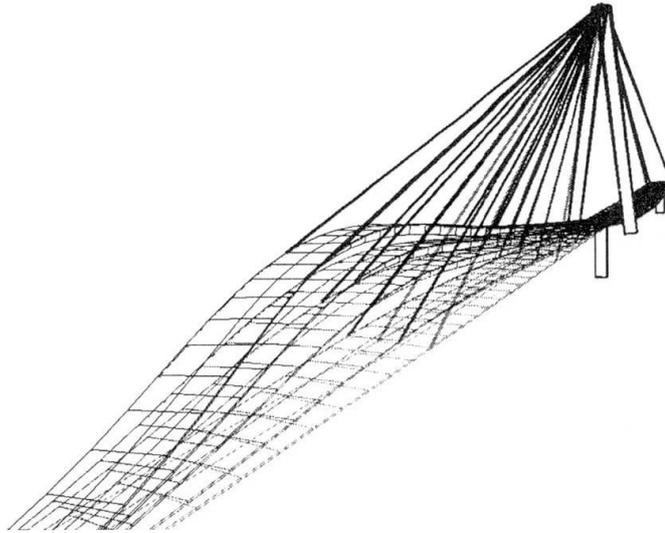
Fig. 1 Eigenmode animated from measurement
