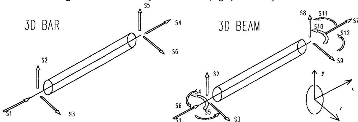
Fig.1: The 3D bar and beam member
