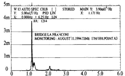
Fig. 8 Monitoring PSD at point 039
