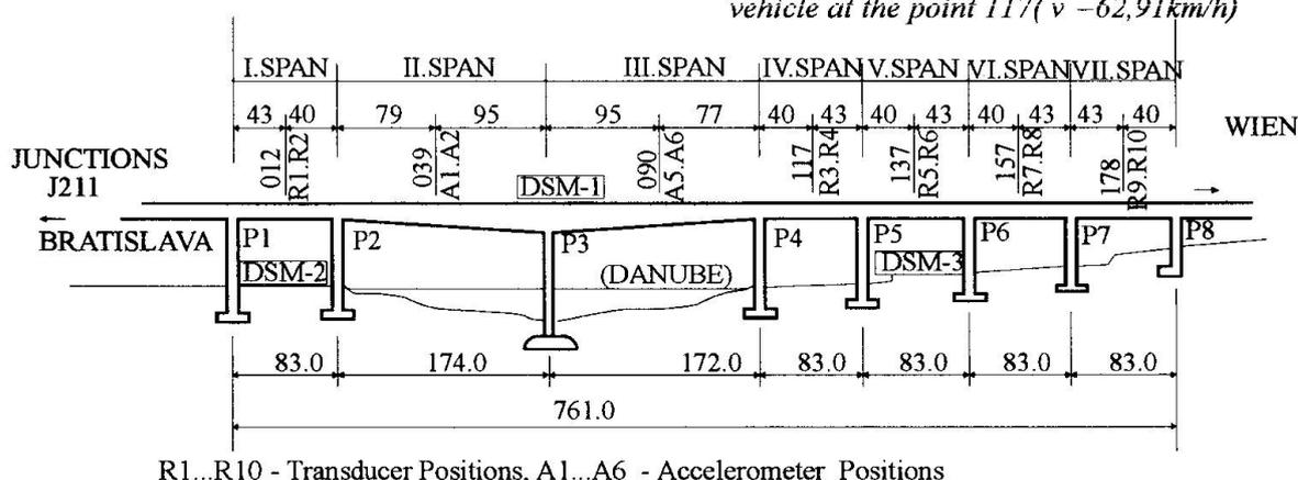
R1...R10 - Transducer Positions, A1...A6 - Accelerometer Positions
