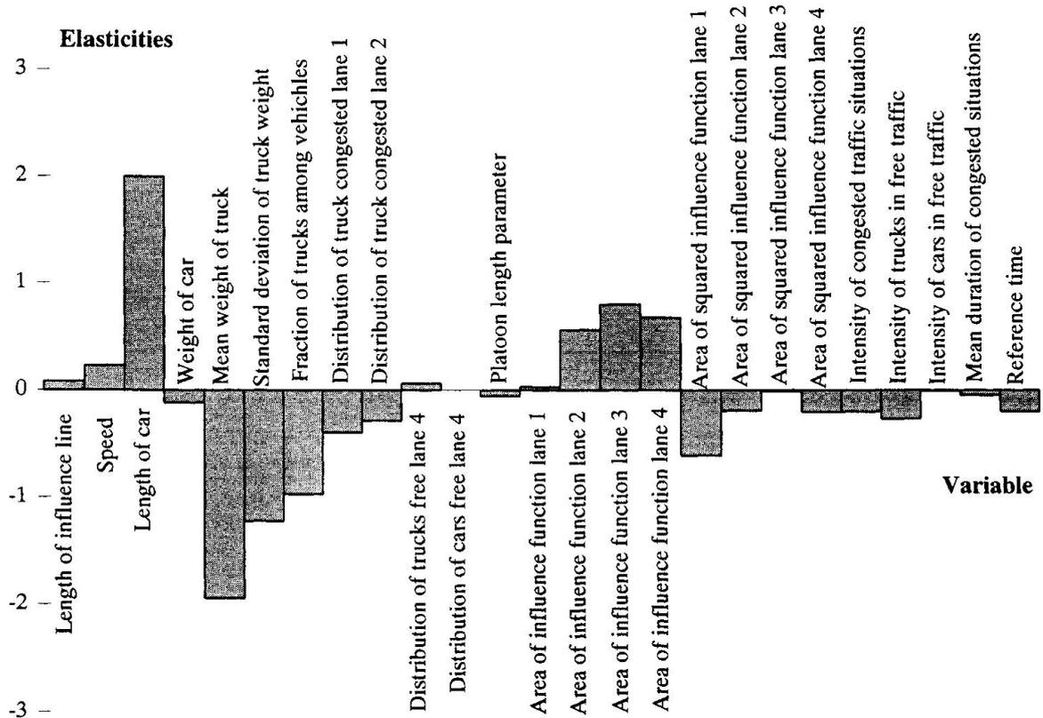
Fig. 3 Sensitivity analysis of the roadway load model.
