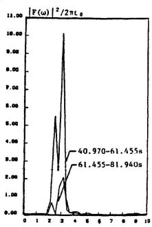
Fig. 3 Acceleration power spectrum of SCT-EW 1985 Mexico earthquake (after Grigoriu et al)
