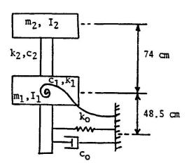
Fig.1 Three-degree model of standing man in the fore and aft mode
