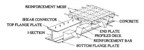
Fig.1 Schematic View Of A Slim Floor Beam
