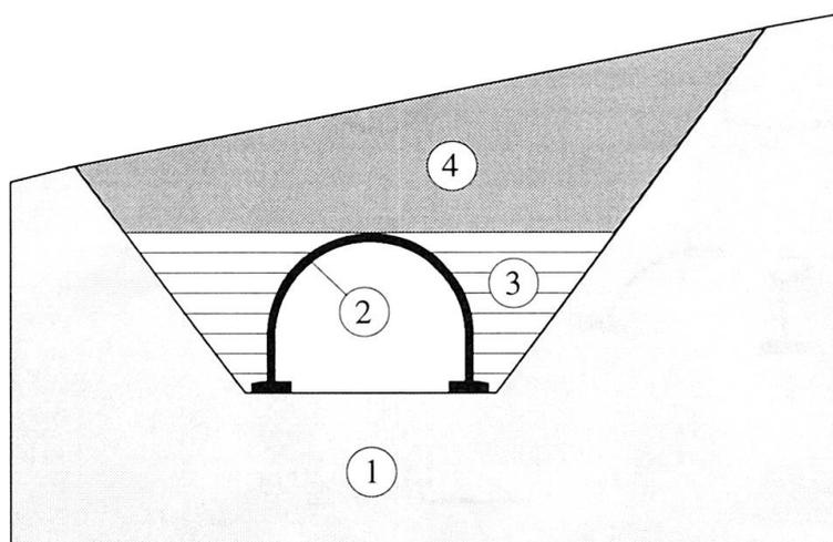
Fig. 5 The structural system for a cut-and-cover tunnel
