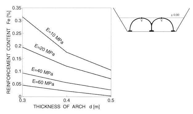
Fig. 19 Lateral backfilling up to the crown. Required reinforcement content (Fe) as a function of chosen values of E and d.
