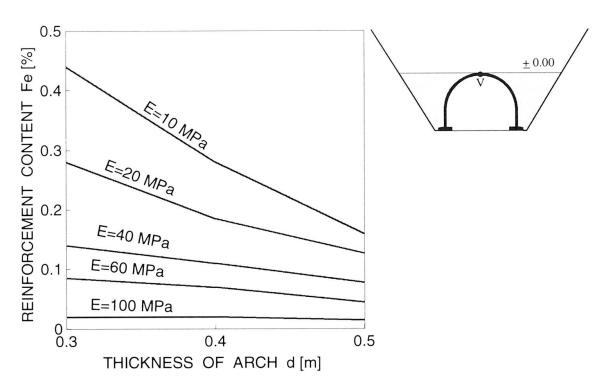
Fig. 15 Lateral backfilling up to the crown. Required reinforcement content (Fe) as a function of chosen values of E and d.
