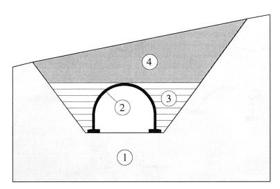
Fig. 5 The structural system for a cut-and-cover tunnel
