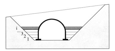
Fig. 8 The simulation of the backfilling stage i
