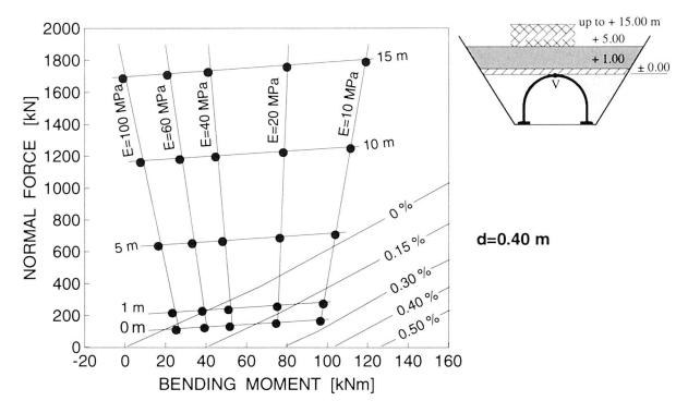
Fig. 13 Interaction diagram M/N for the crown V for the backfilling stage to the crown with backfilling increments of 5, 10 and 15 m Thickness of arch 0.40 m (reinforcement content in %)
