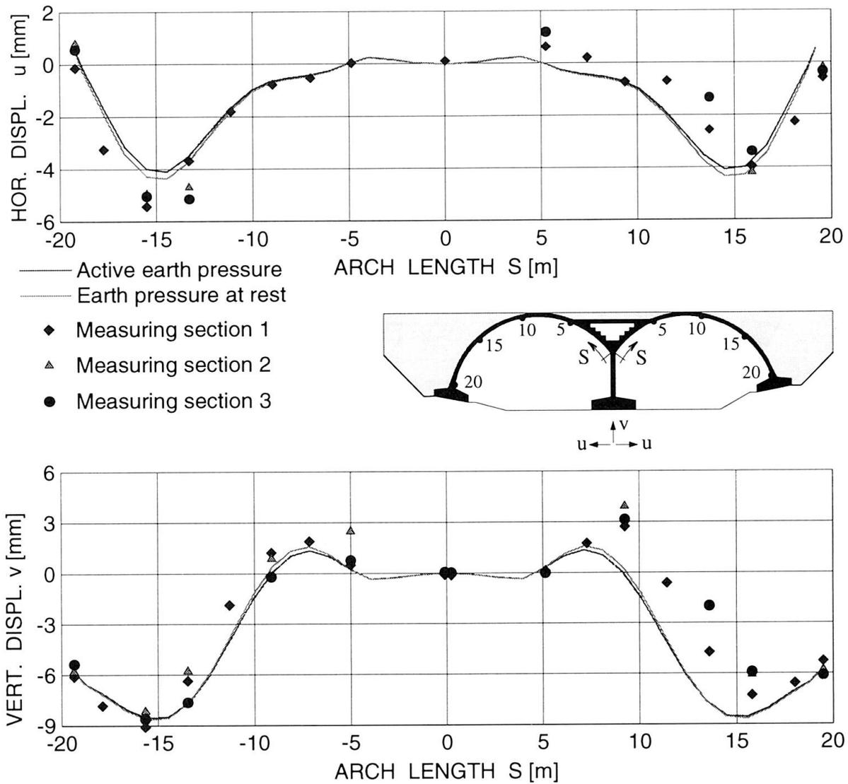
Fig. 10 Brünnen Tunnel: Comparison of measured displacement components  $(u, v)$  in discrete points with the calculated bending deflection curve
