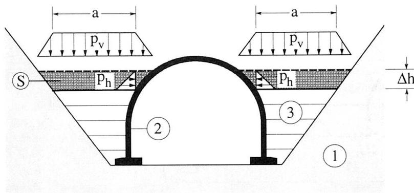
Fig. 6 The layer *S* during compaction
