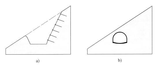
Fig. 3 Cut-and-cover tunnel in sloping ground a) Excavation and support of slope b) Construction of tunnel arch and backfilling
