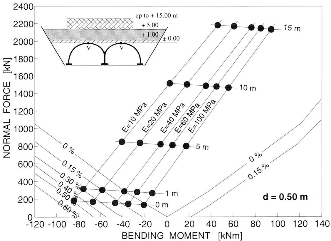
Fig. 18 Interaction diagram  $M/N$  for the crown  $V$  for the backfilling stage to the crown with backfilling increments of 5, 10 and 15 m
