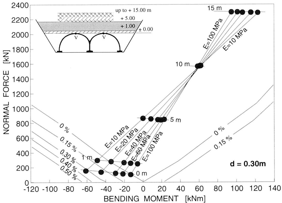
Fig. 17 Interaction diagram  $M/N$  for the crown V for the backfilling stage to the crown with backfilling increments of 5, 10 and 15 m
