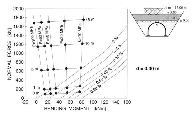
Fig. 12 Interaction diagram M/N for the crown V for the backfilling stage to the crown with backfilling increments of 5, 10 and 15 m
