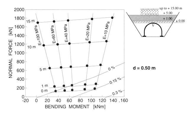
Fig. 14 Interaction diagram M/N for crown V at the backfilling stage to the crown and backfilling increments of 5, 10 and 15 m.
