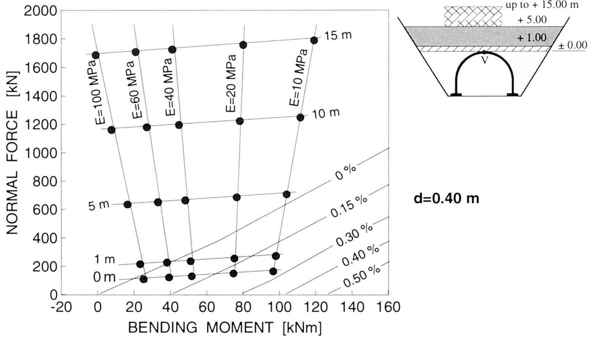
Fig. 13 Interaction diagram M/N for the crown V for the backfilling stage to the crown with backfilling increments of 5, 10 and 15 m
