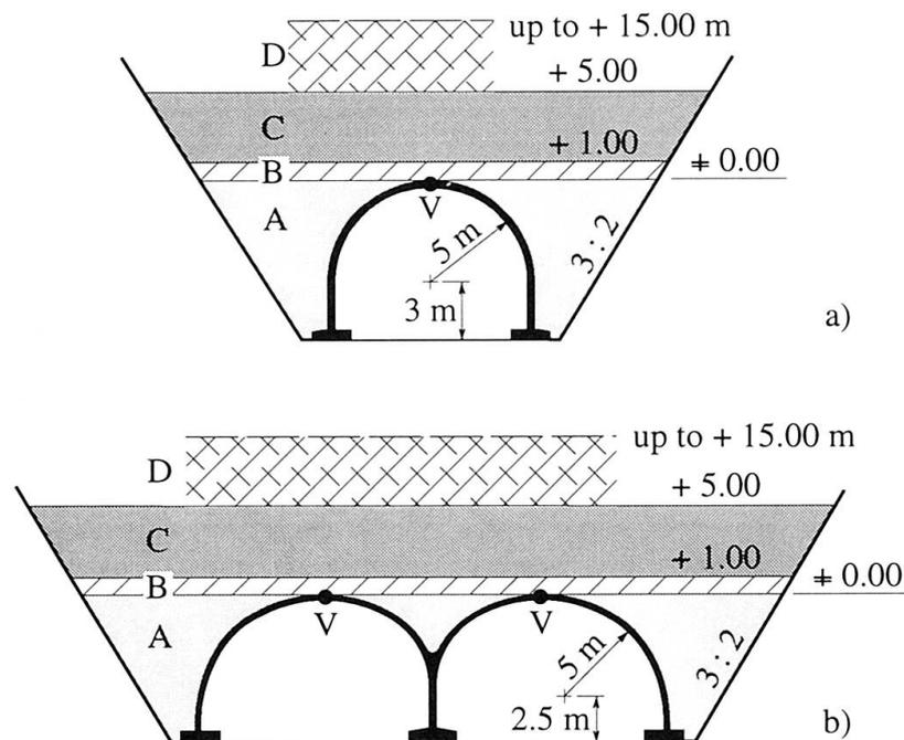
Fig. 11 Geometry of the profile and the computed backfilling stages A to D. The design charts refer to the cross-section at the crown of the arch (point V).
