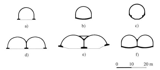
Fig. 4 Typical profiles in traffic tunnels
