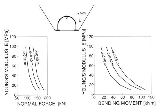
Fig. 16 The internal moments and forces M and N as a function of the Young's modulus E of the backfilling and the thickness of the arch d
