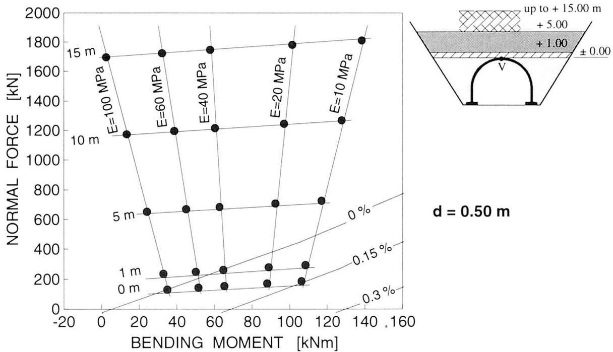
Fig. 14 Interaction diagram M/N for crown V at the backfilling stage to the crown and backfilling increments of 5, 10 and 15 m.
