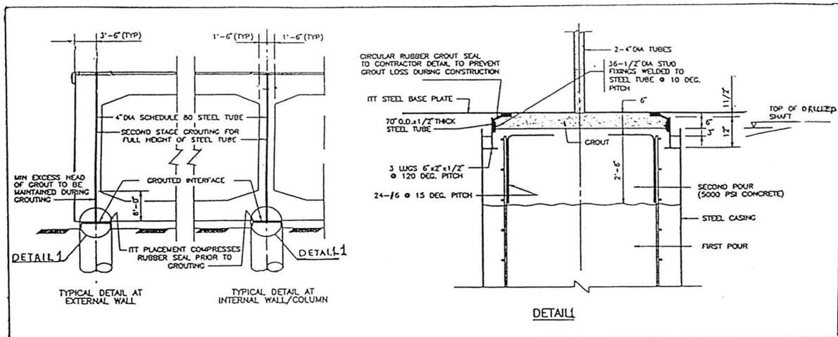
Figure 3. ITT - Drilled shaft Connection
