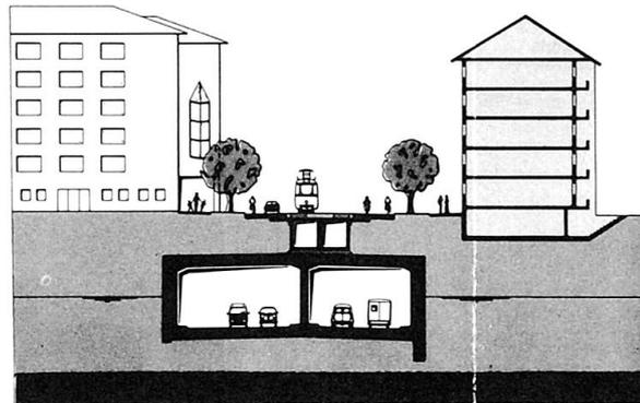
Fig. 3 Tunnel 'Horburg West': Typical Cross Section
