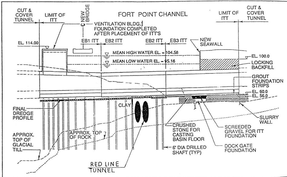
Figure 2. Longitudinal section I-90 EB in the FPC
