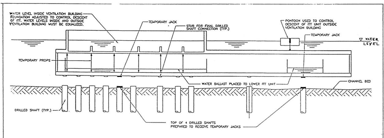
Figure 5. Immersion of the ITT with snorkel
