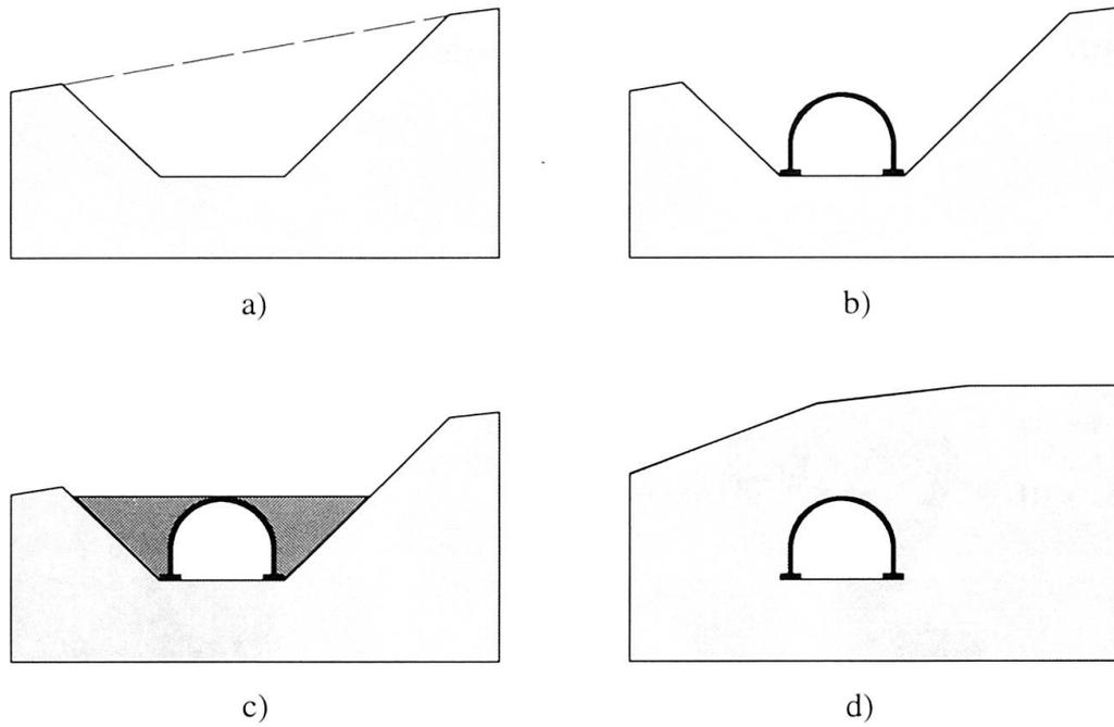
Fig. 1 The different construction stages of a typical cut-and-cover tunnel
