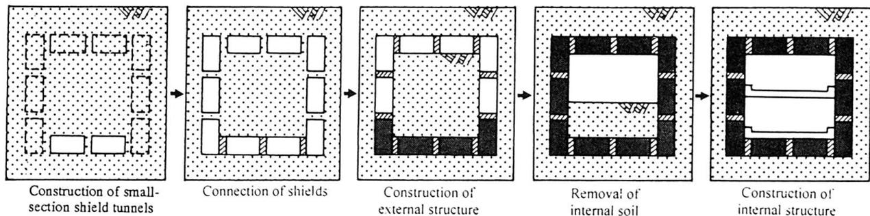
Fig. 2 Construction procedure according to the MMST method
