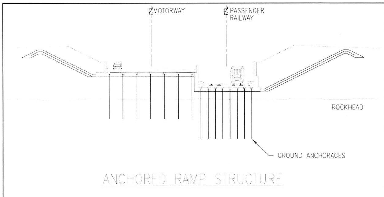
Figure 1: Typical Cross Section through ramps
