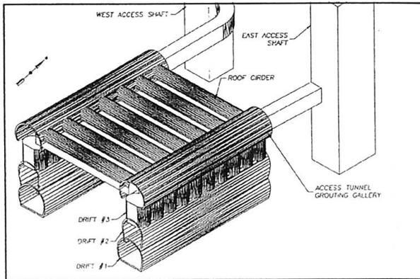
Figure 4. Conceptual Layout of Underpinning of South Station
