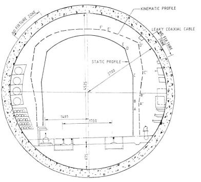
Fig. 6 Typical Cross-section of Tunnel in Rock Tunneling
