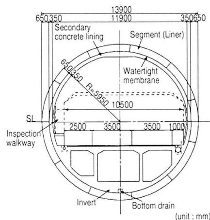
Fig. 6 Tunnel cross section and traffic lanes
