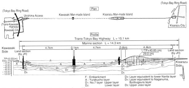
Fig. 2 Project plan and geological profile
