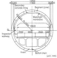
Fig. 6 Tunnel cross section and traffic lanes
