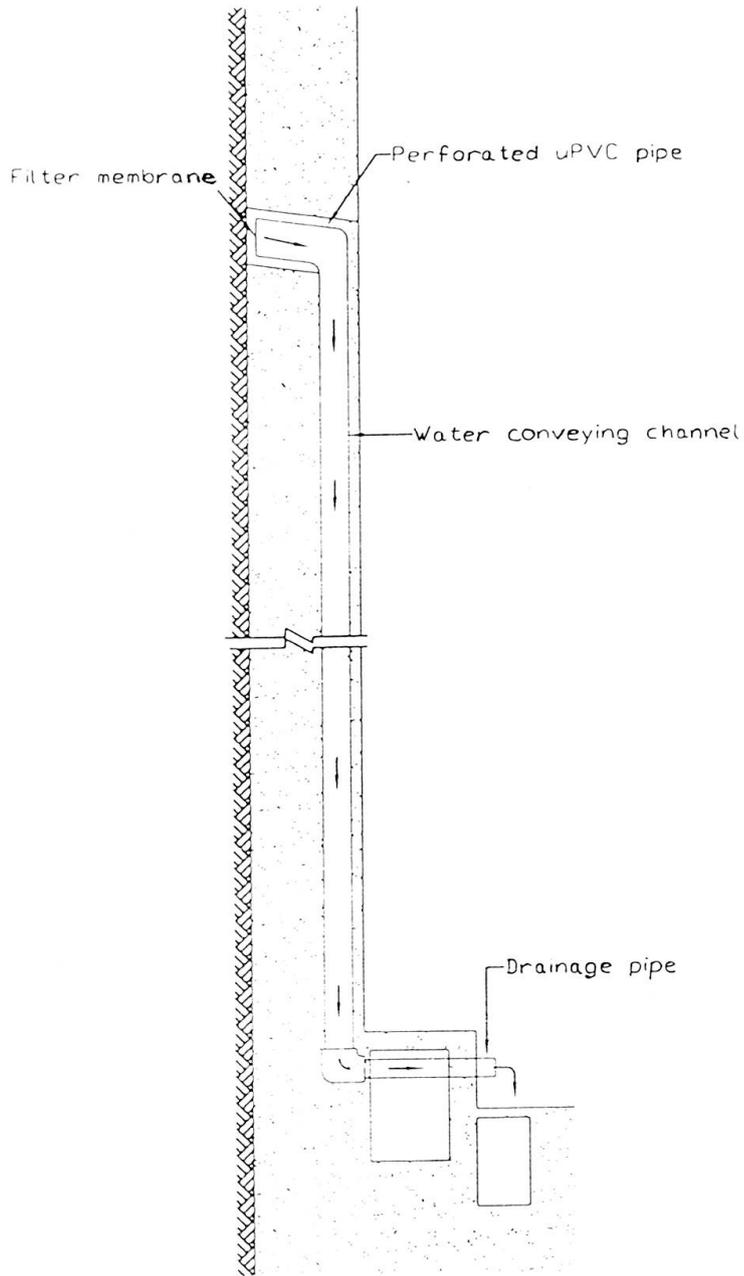
Fig. 6 Section through expansion joint showing drainage system
