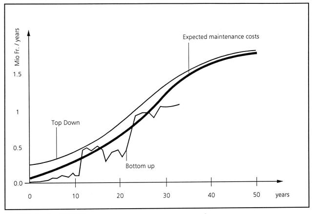
Fig. 3 Prediction of the costs of maintenance with both approaches
