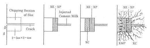
Figure 2. Rough Sketch of Triple Plugging Method
