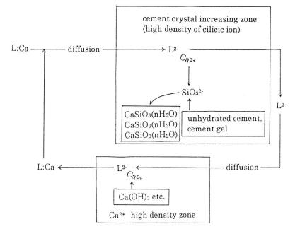
Figure 1. Basic Mechanism of Cement Crystal Increasing
