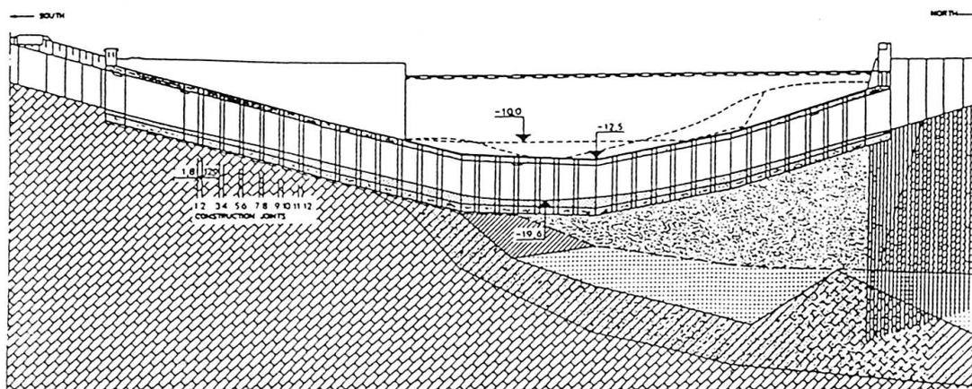
The units were waterproofed with a 2 mm butyl membrane which, as described in the introduction, has never been fully effective.
