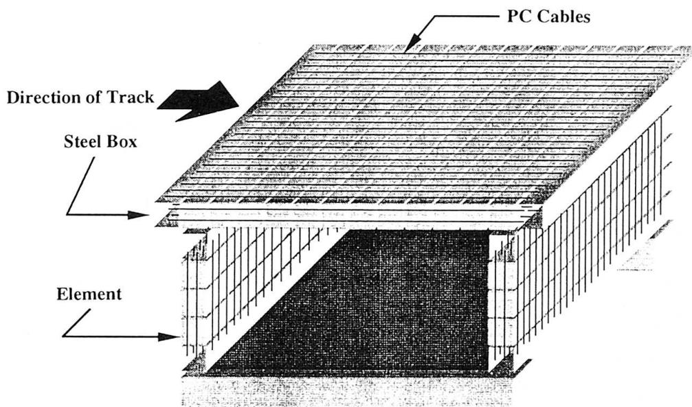
Fig. 2 Conceptual Diagram of Pre-cast Block Lateral Tightening Method
