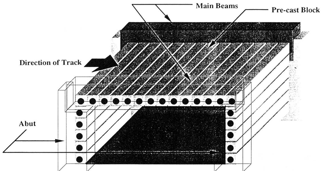
Fig. 1 Conceptual Diagram of Pre-cast Block Method
