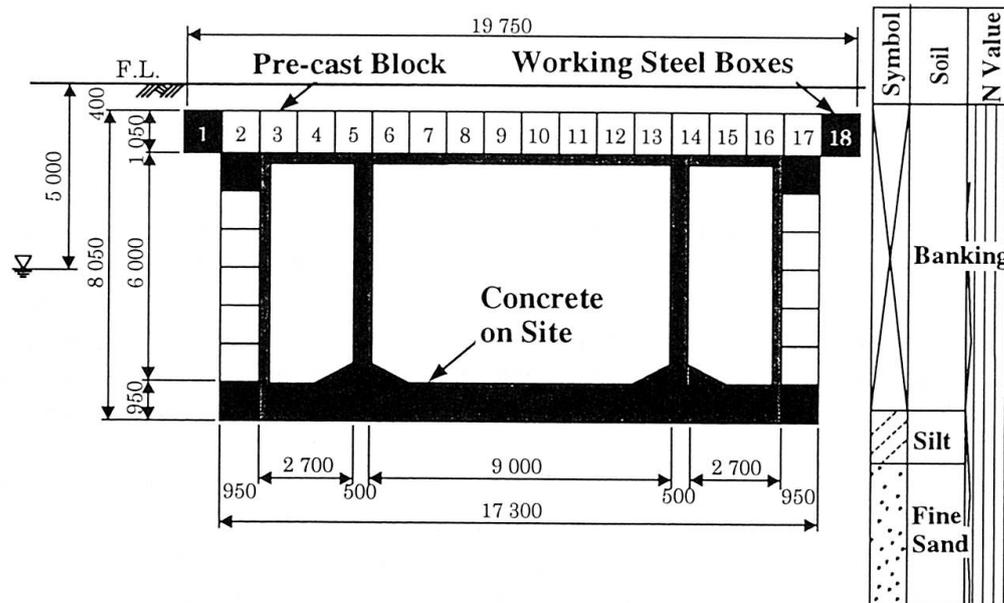
Fig. 5 Sectional View of Slab Beam Type
