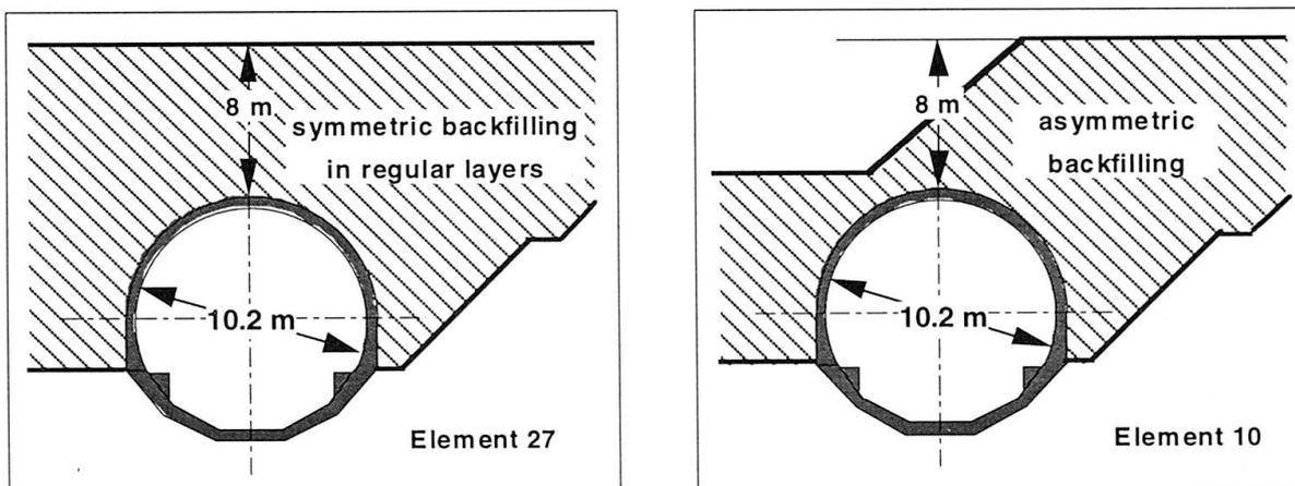
Fig. 6 Correct symmetric backfilling (Element 27) and incorrect backfilling (Element 10)
