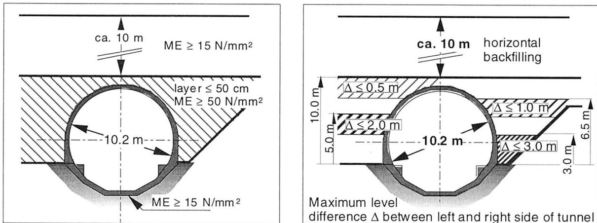
Fig. 3 The backfill instructions for the contractor
