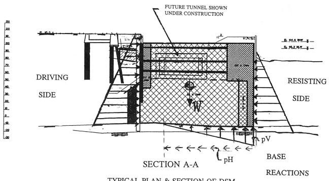
TYPICAL PLAN & SECTION OF DSM FIGURE 4
