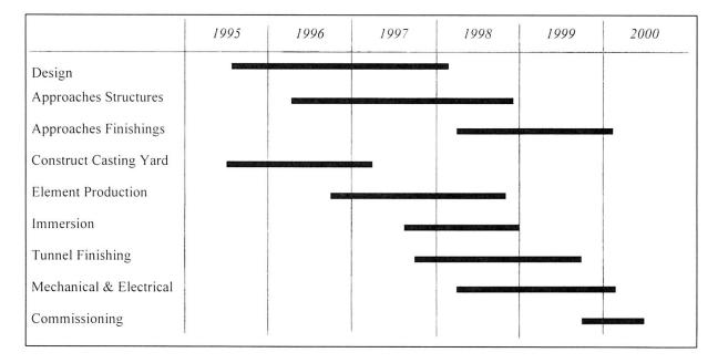
Fig. 1 ØTC time schedule for the tunnel
