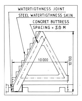
Figure 4. Sliding gate cross section
