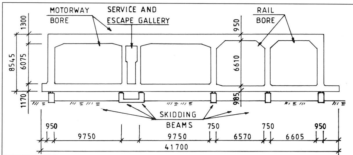
Figure 3. Cross section through tunnel and skidding beams.
