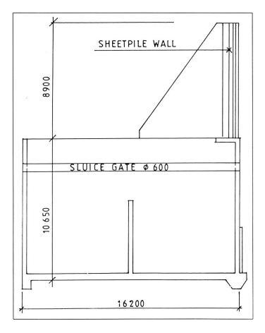
Figure 5. Floating gate cross section
