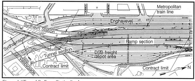
Figure 1 "Tunnel Sydhavn Station" -plan
