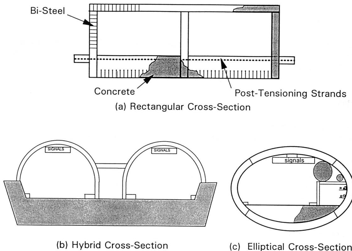
Fig. 4 Immersed tunnel cross-sections possible using Bi-Steel
