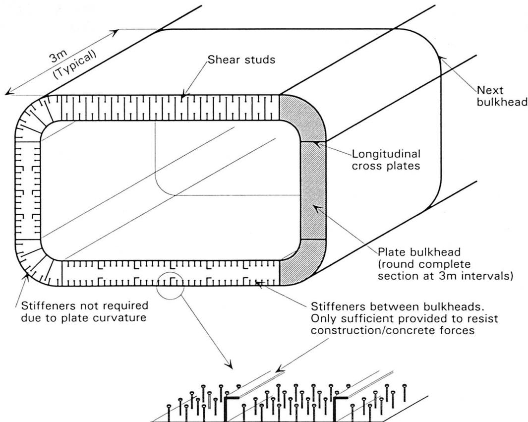
Fig.1 Steel-Concrete-Steel (SCS) construction using shear studs.
