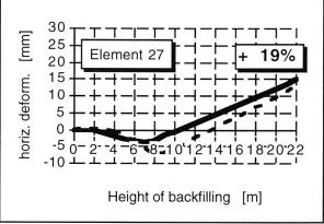
Fig. 7 Difference between calculation (dotted line) and measurement of the vertical and horizontal deformations at element 27
