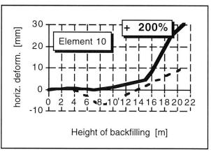
Fig. 8 Difference between calculation (dotted line) and measurement of the vertical and horizontal deformations at element 10
