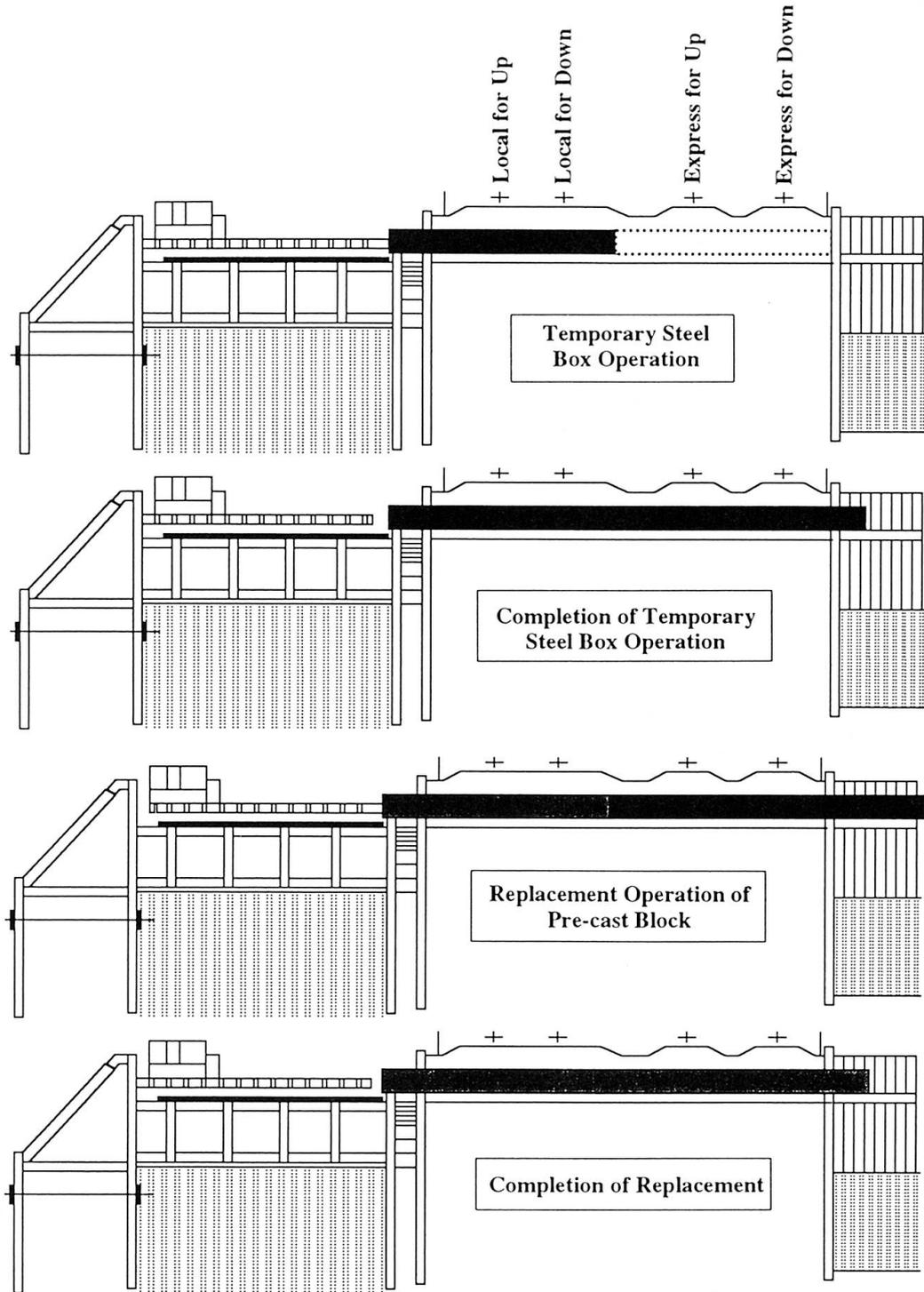
Fig. 8 Sequence of Replacement Construction
