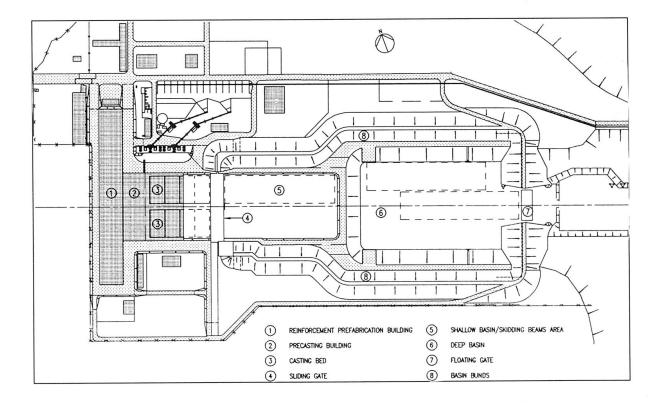
Figure 2. Plan of construction facility.
