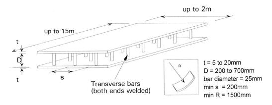
Fig. 2 Initial production range of Bi-Steel panels
