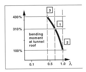
Fig. 2 Different shapes of the l\u00e4value and its influence on the bending moment at the tunnel roof
