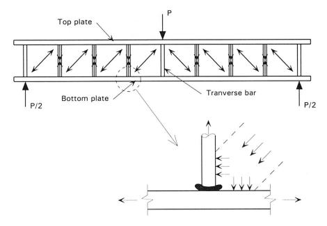
Fig. 3 Diagram showing how Bi-Steel may be visualised as carrying load
