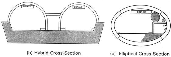
Fig. 4 Immersed tunnel cross-sections possible using Bi-Steel
