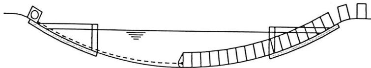
3) Flood approach works. Progressively pull tunnel through.
