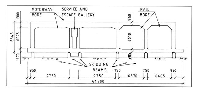
Figure 3. Cross section through tunnel and skidding beams.
