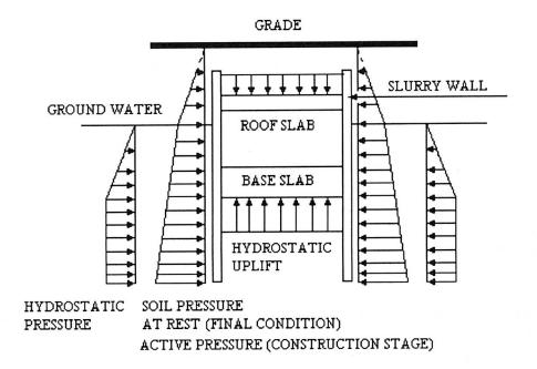
Figure 2. Typical Tunnel Load Diagram
