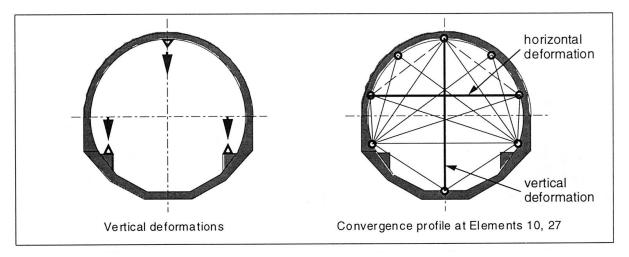
Fig. 5 Cross sections through the tunnel tubes with the measuring points for vertical deformation measurement and convergence profile
