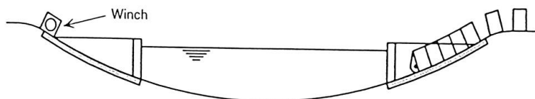
2) Dredge channel. Assemble elements on slipway. Weld together concrete fill.
