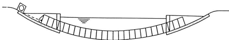
4) Seal off at waterbond. Drain approach works. Remove winch.
