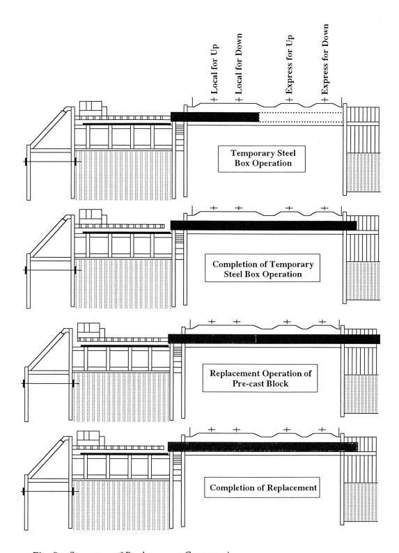
Fig. 8 Sequence of Replacement Construction
