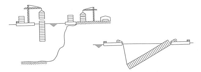
Fig. 5 Construction of tunnel elements in deep water
