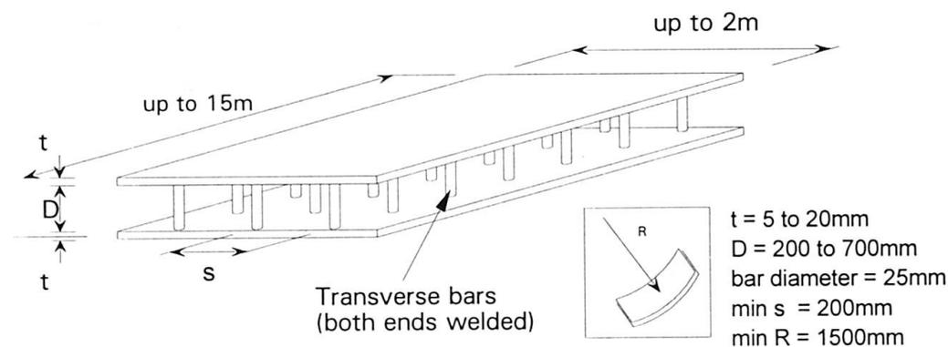
Fig. 2 Initial production range of Bi-Steel panels
