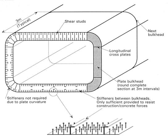
Fig. 1 Steel-Concrete-Steel (SCS) construction using shear studs.
