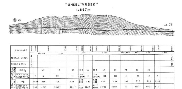
Estimated longitudinal profile of the Vršek tunnel with separate presentation of Figure 2 hazard and specific risk
